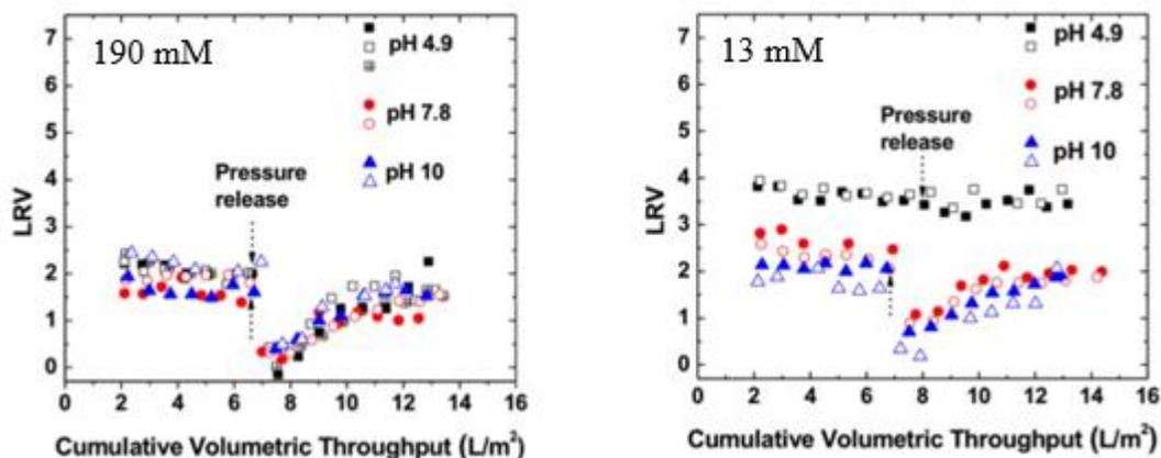
Figure 3: Virus Retention in Pressure Release Filtration Experiments
