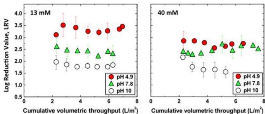
Figure 2: Virus Retention in Constant Pressure Filtration Experiments
