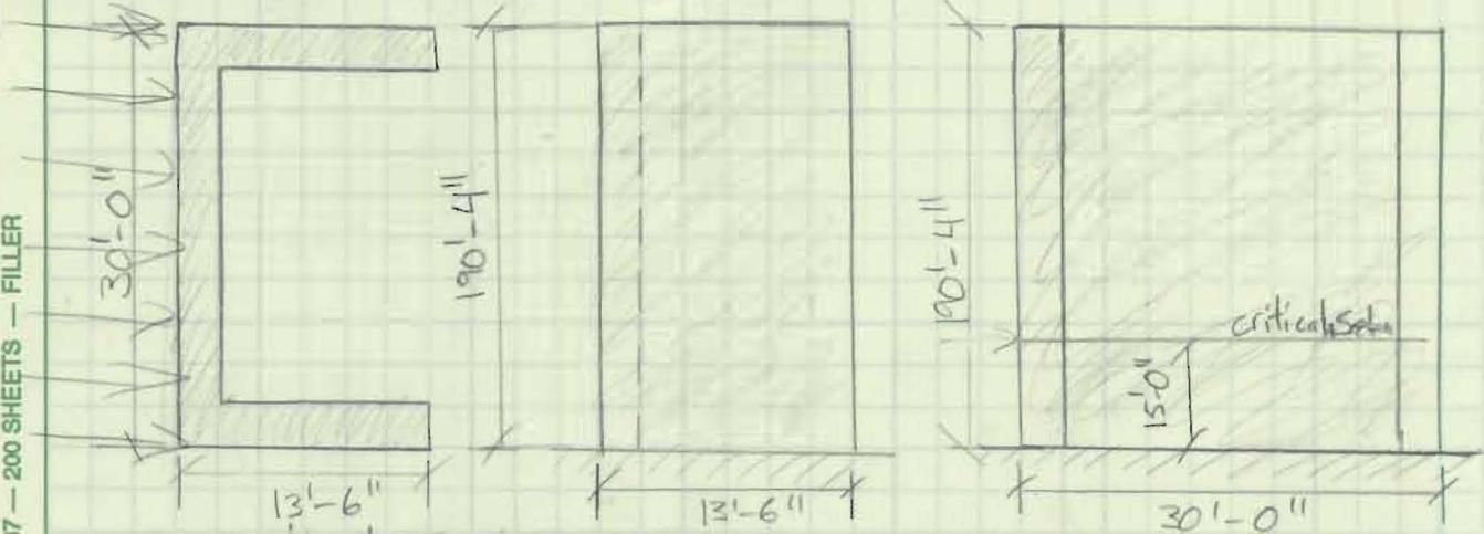
Critical Section for 30'-0" span
