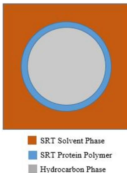
**Figure 7. Cross Section of an SRT-coated Colloid Particle**
