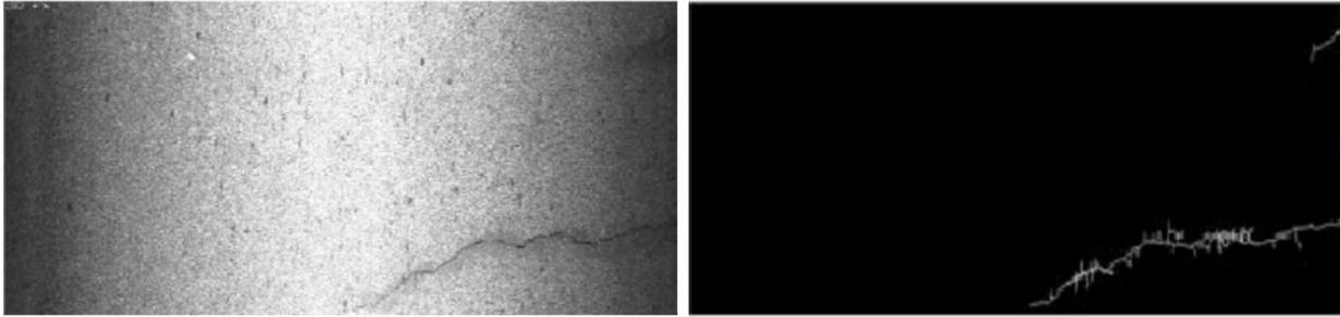
Figure 15: Original grayscale image with crack (left), and binary image after processing (right) [23]
