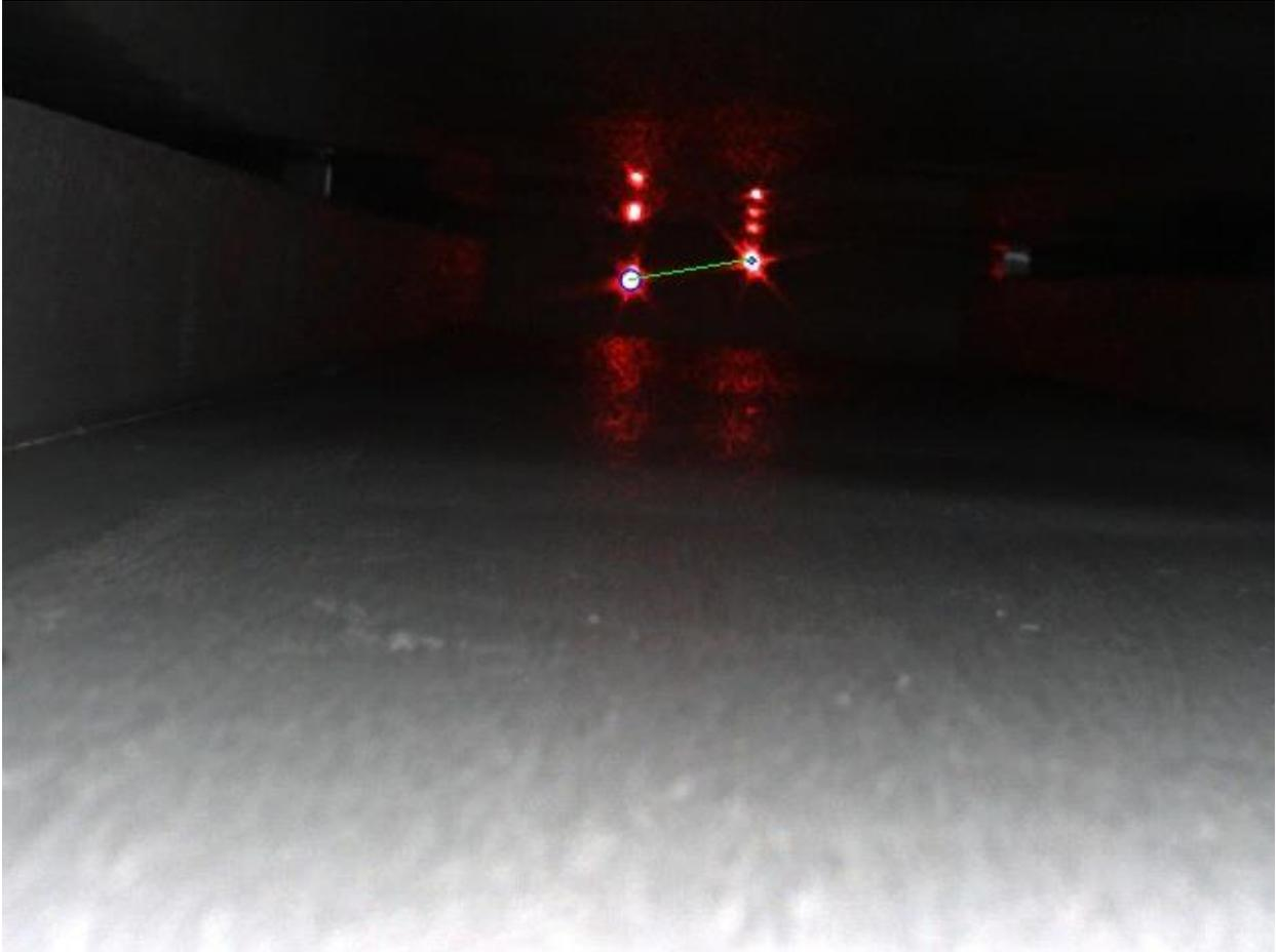
**Figure 28:** View from the robot inside the mockup, the green line illustrates the distance used to measure laser separation
