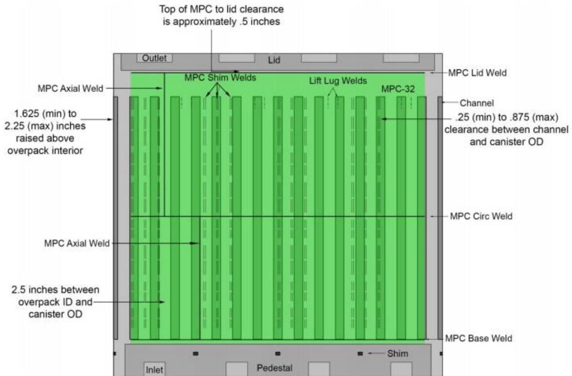
Figure 2: Unrolled view of the air gap between the MPC and overpack [5]
