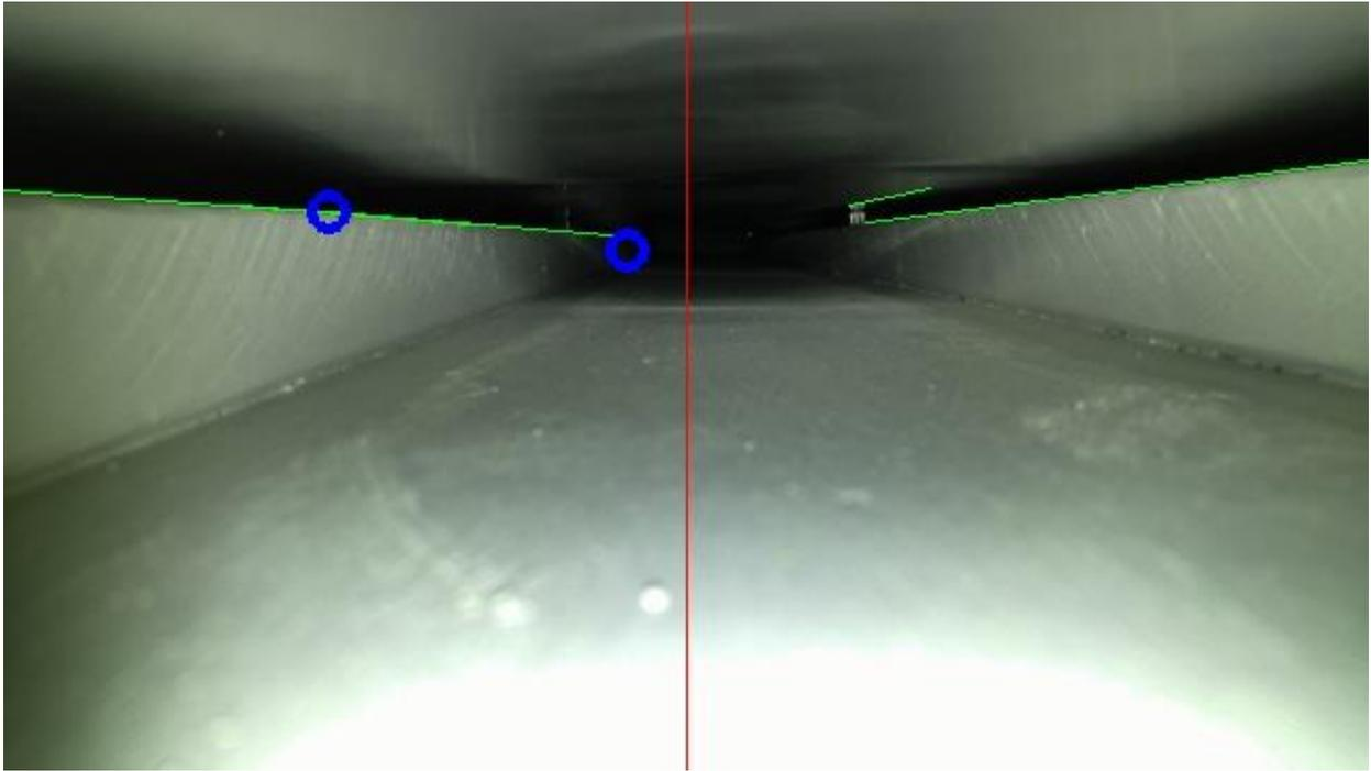
Figure 32: Edge detection as applied to an image captured by secondary test equipment inside the mockup (for an explanation of the annotations, see Figure 23)
