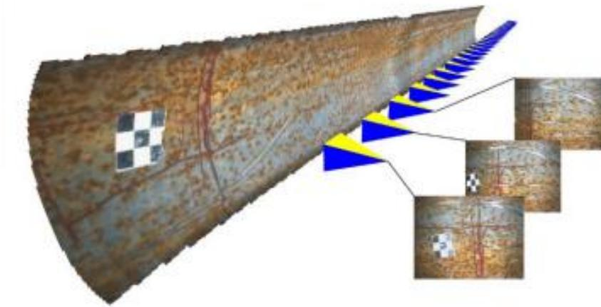
Figure 14: Render of pipe interior created from camera imagery and odometric data [22]
