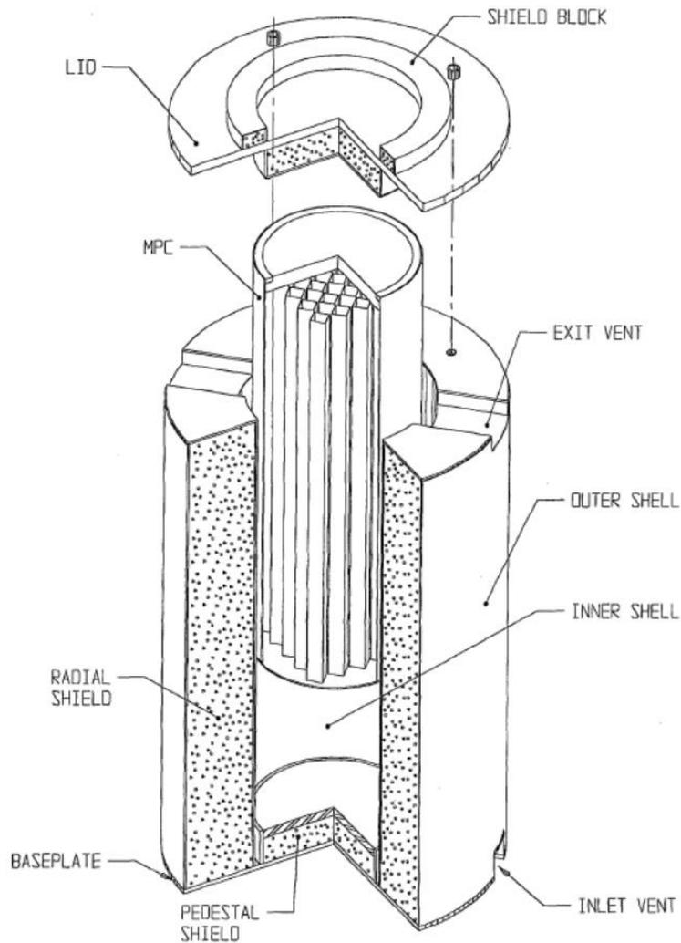
Figure 1: Exploded view of a Holtec International HI-STORM 100 storage system [4]
