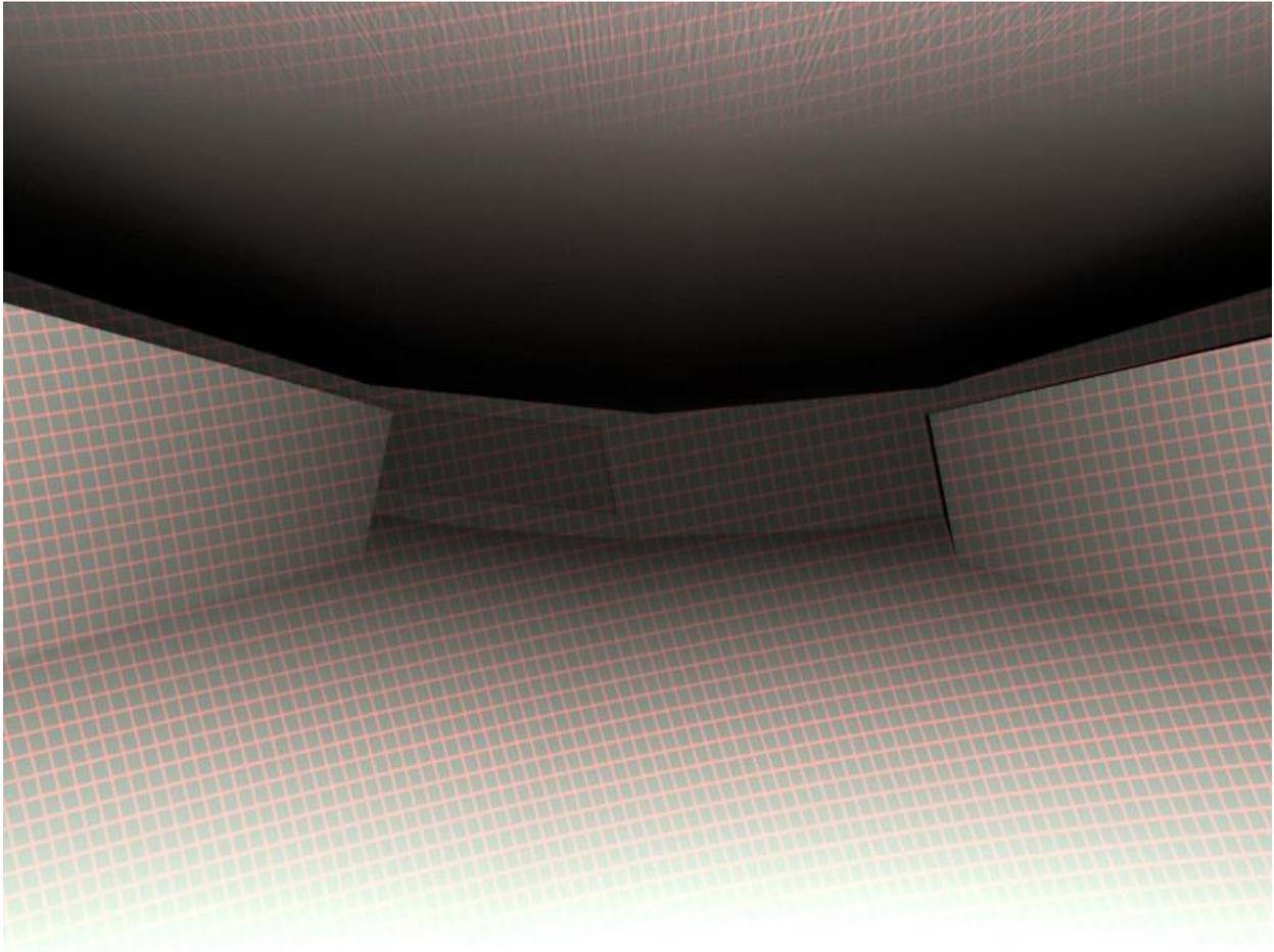
Figure 18: A grid pattern projected by a laser onto the simulated channel
