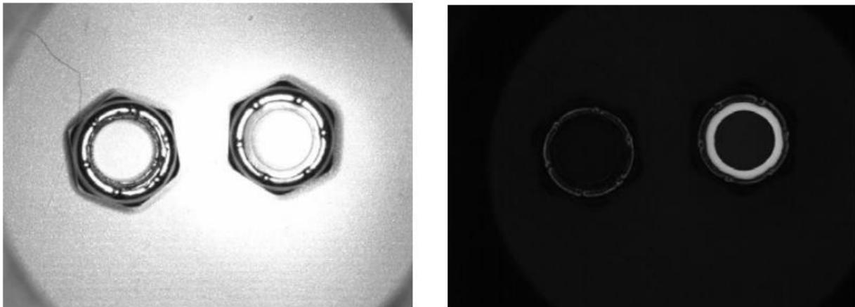
Figure 13: A red (>510nm) filter blocks ambient light (right), showing the UV reflected by the nylon ring [21]
