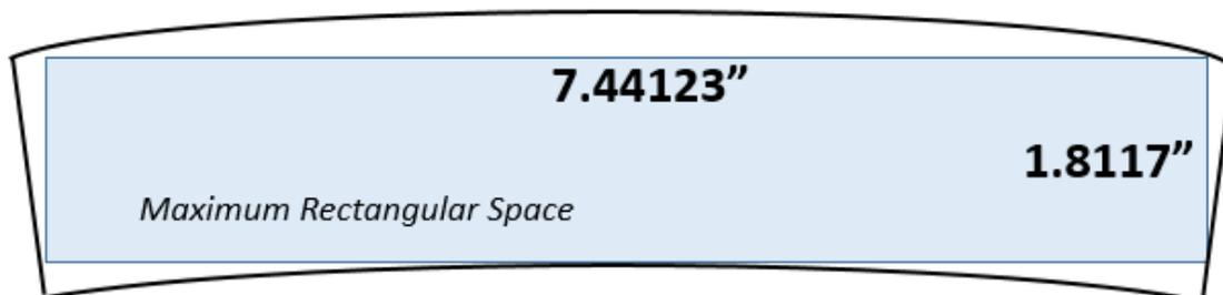
Figure 3: Rectangle as constrained by channel dimensions [11]
