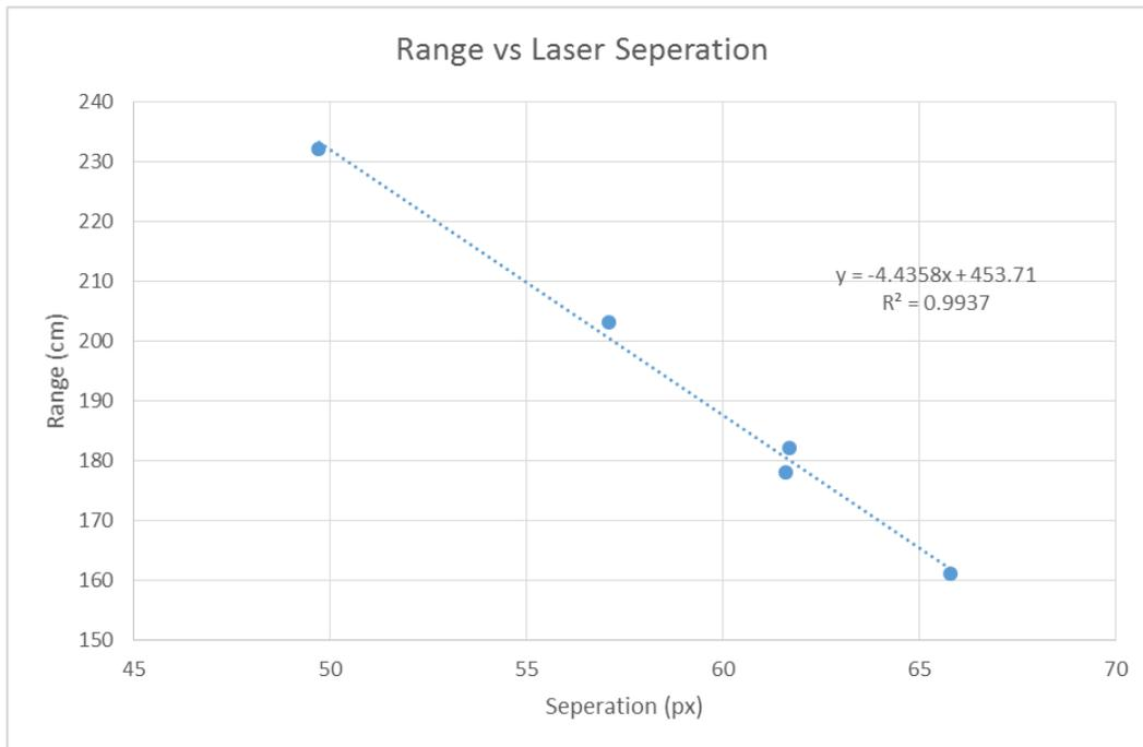
Figure 29: Calibration curve of the relationship between laser separation and range
