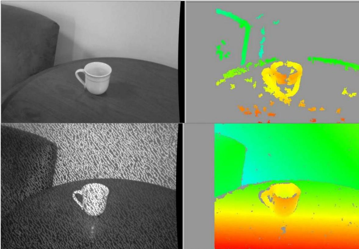
Figure 11: Scene and disparity map under normal conditions (top), and with projected texture (bottom) [18]
