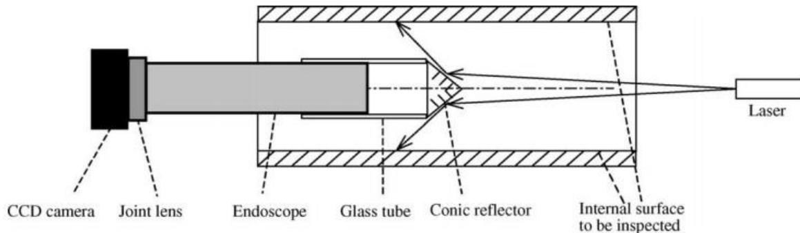
Figure 12: A system for inspecting pipe interiors using circle structured light [20]
