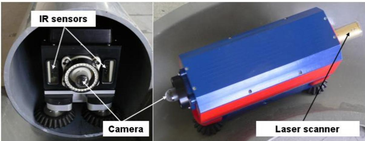
Figure 6: The KANTARO sewer inspection robot [14]
