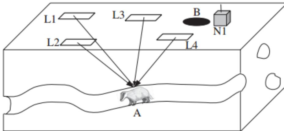
**Figure 9: A magneto-inductive tracking system showing transmitters (L1-L4), receiver (A), and a basestation (N1) near the tunnel exit (B) [16]**
