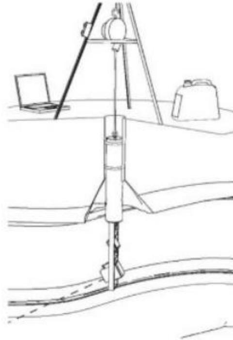
Figure 7: The process of using a BDL for void inspection [15]
