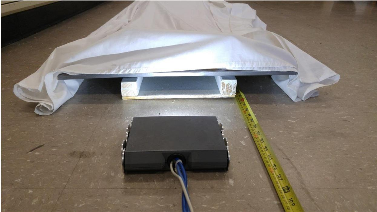
**Figure 27: Robot prototype at entrance to mockup (cloth in place to block ambient light)**
