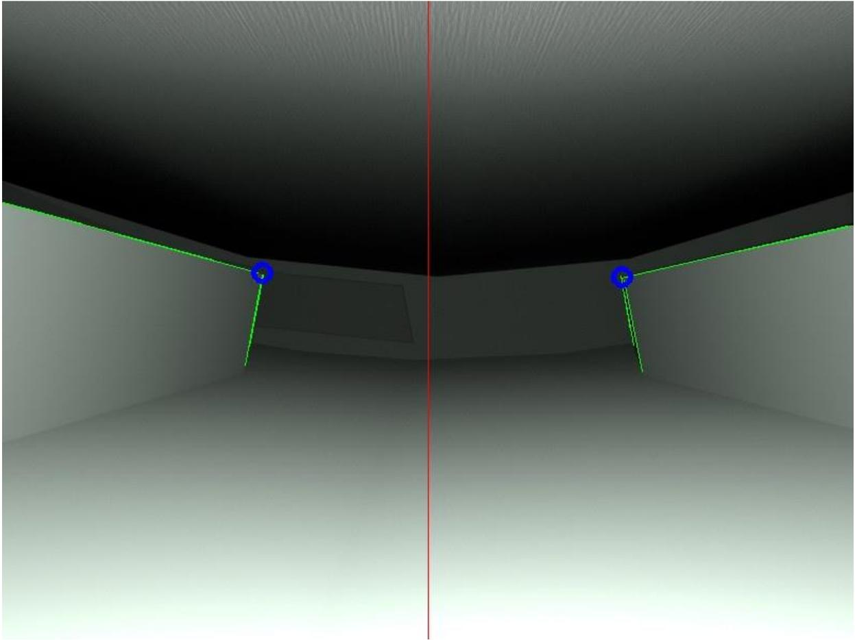
Figure 23: Two blue circles highlight the identified intersections, green lines show the extracted edges, and a red line shows where the image is split into left and right halves
