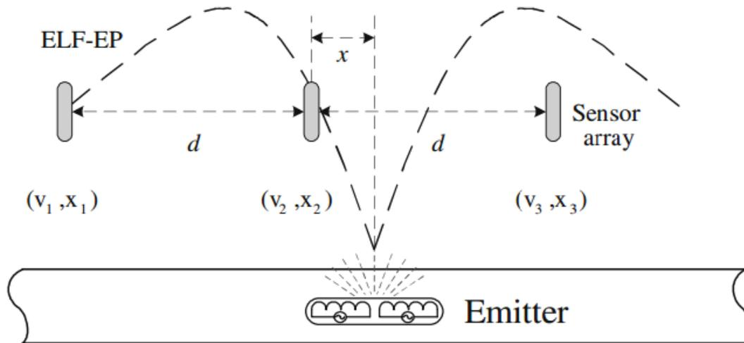
Figure 10: Localization by measuring the strength of ELF pulses [17]
