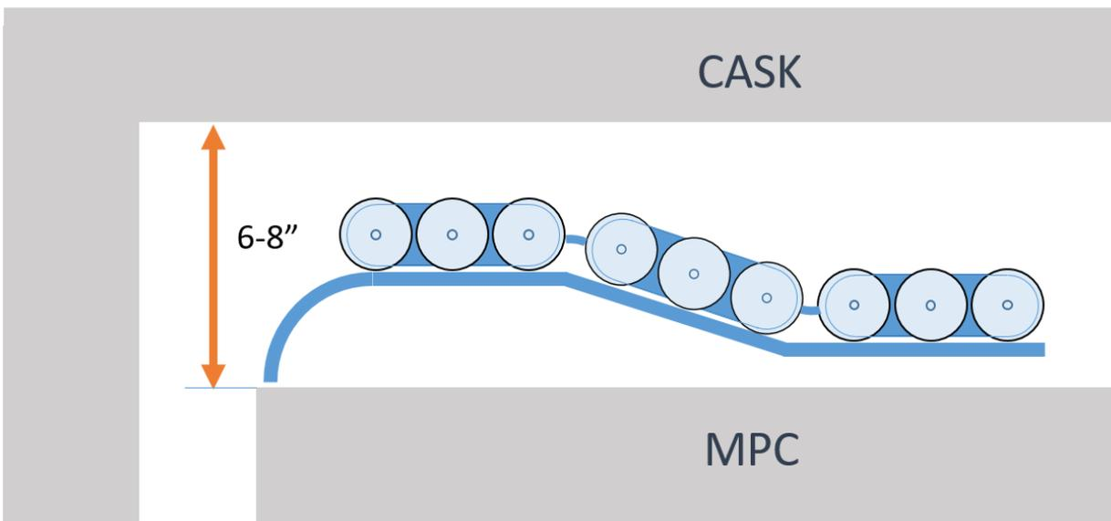
Figure 4: Concept of the inspection robot resting on top the MPC [11]
