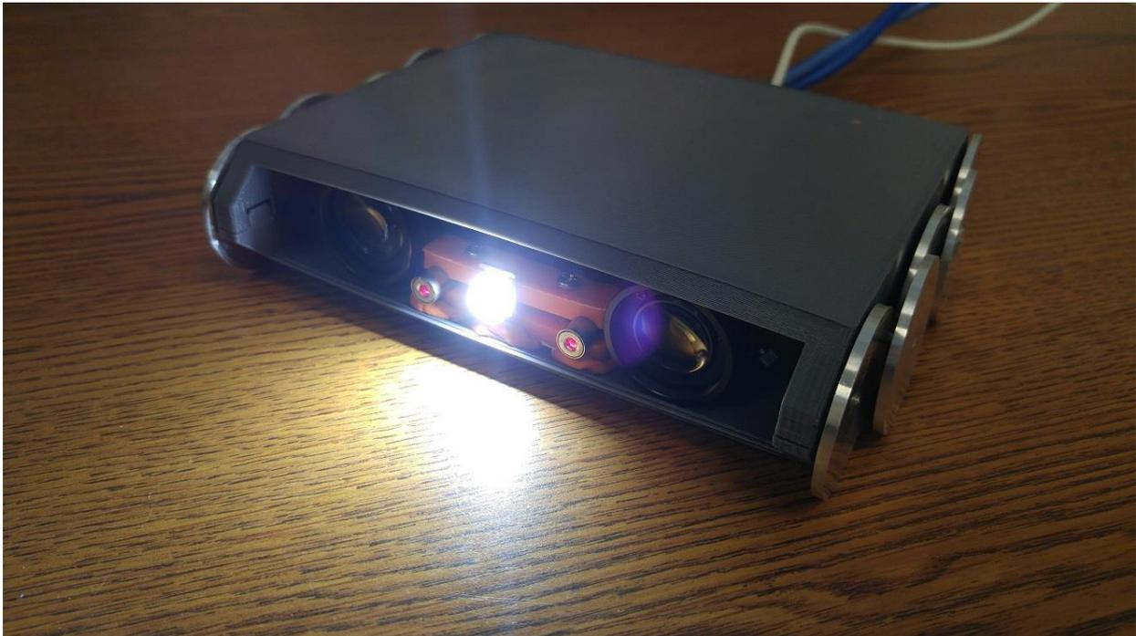
Figure 26: Inspection robot prototype “Splinter” with LED lamp and lasers
