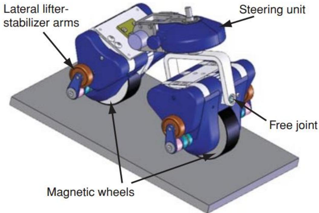
Figure 5: Design of the MagneBike inspection robot [12]
