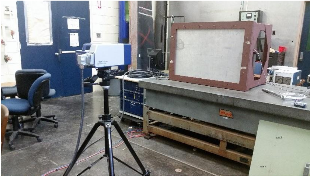
Figure 9. Laser Doppler vibrometer scanning head pointing at a plate that is mounted on a steel frame.
