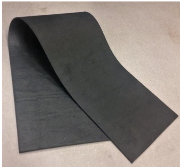
Figure 5. Viscoelastic damping material used in the experiment.
