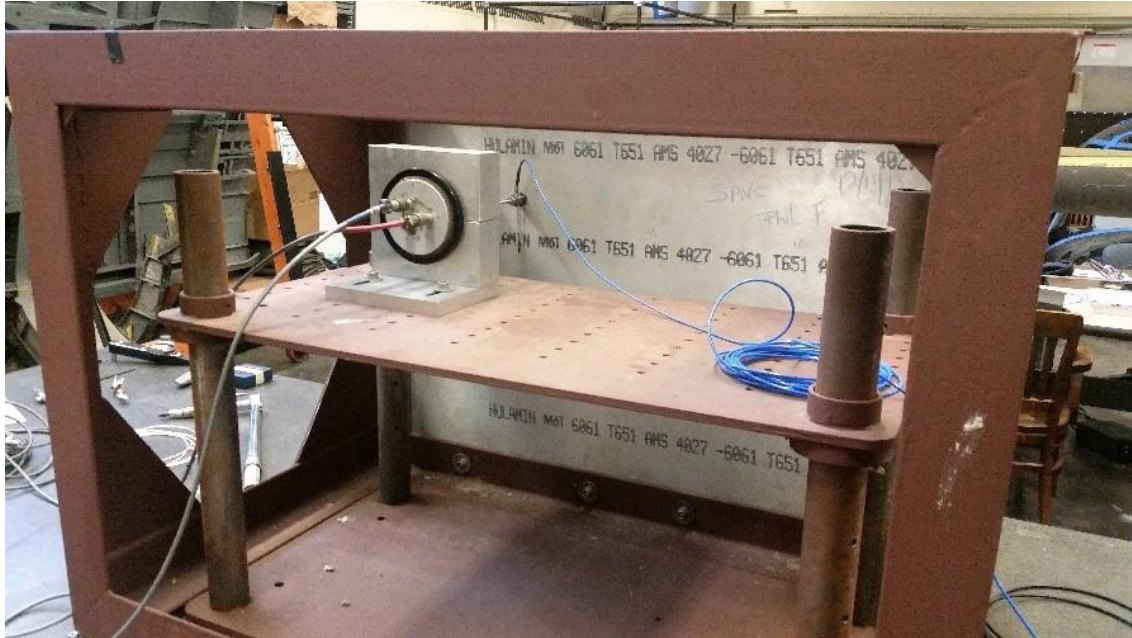
Figure 6. Uniform plate mounted in a steel frame with shakers attached by an impedance head.
