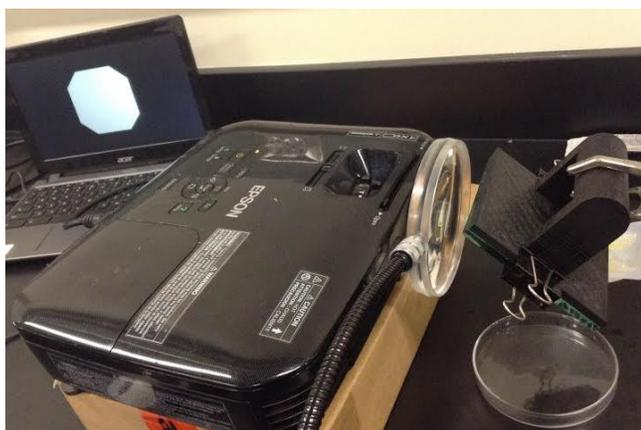
**Figure 15: An EPSON proctor, mirror, and lense creates a remedial DLP system.**
