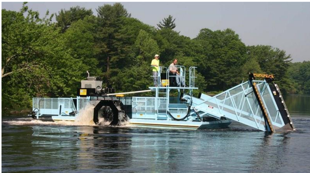
Figure 6: An operating mechanical skimmer ( www.aquarius-systems.com ).
