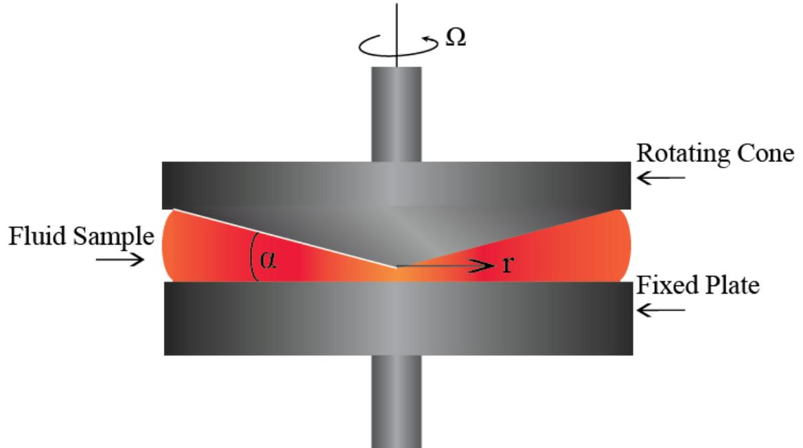
**Figure 2-5. Depiction of Cone-Plate Viscometer.** This instrumentation consists of a 1-degree rotating cone creating a uniform shear field across the entire fluid sample.
