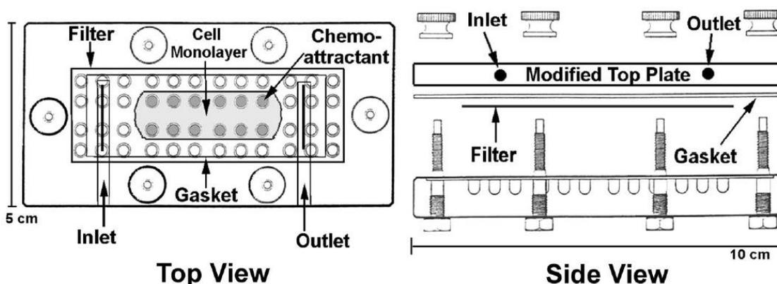
**Figure 2-6. Top and Side Views of the Chemotactic Flow Migration Chamber<sup>40</sup>.** This apparatus consists of a modified chemotactic boyden chamber assay with two polycarbonate plates separated by a silicon gasket. Beneath the gasket is a porous polycarbonate filter with an endothelial monolayer coated with fibronectin.
