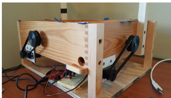
Figure 5 Two Independent Servo motors and control mechanisms
