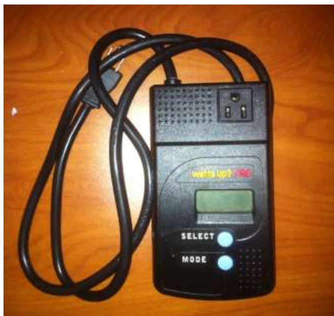
Figure 2-1: Watts up? PRO kilowatt meter used to collect energy consumption data
