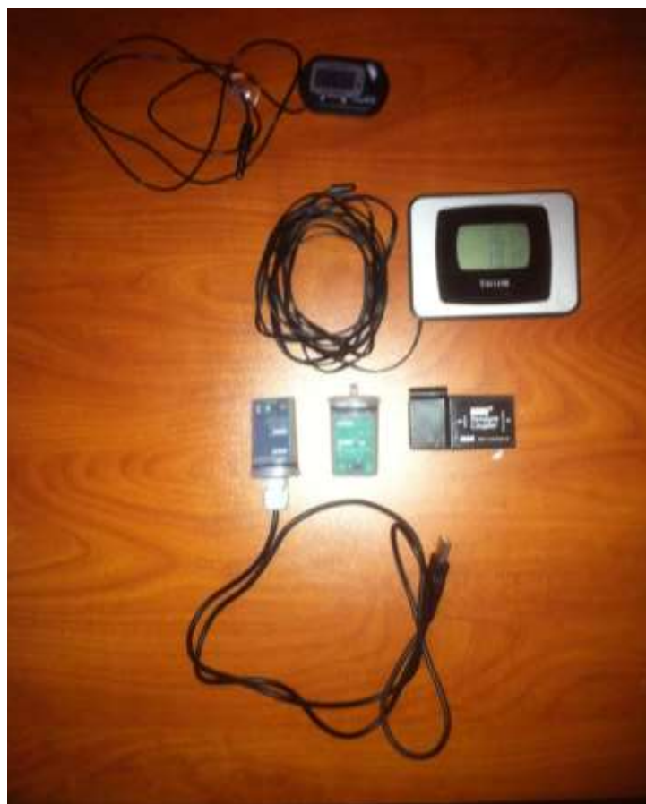
Figure 2-2: HOBOWare temperature sensor and thermometers used to collect temperature data
