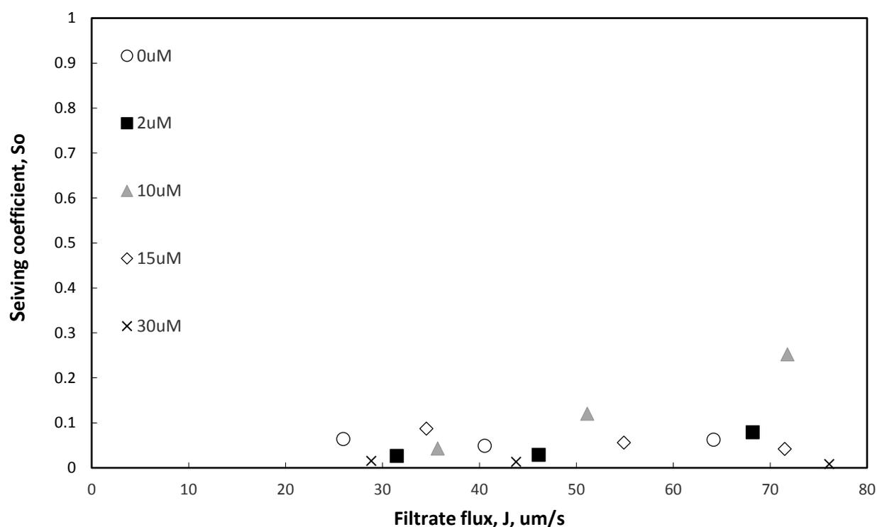
**Figure 6.** Sieving coefficient for open-circular plasmid in 10 mM NaCl TE buffer at different spermine concentrations.
