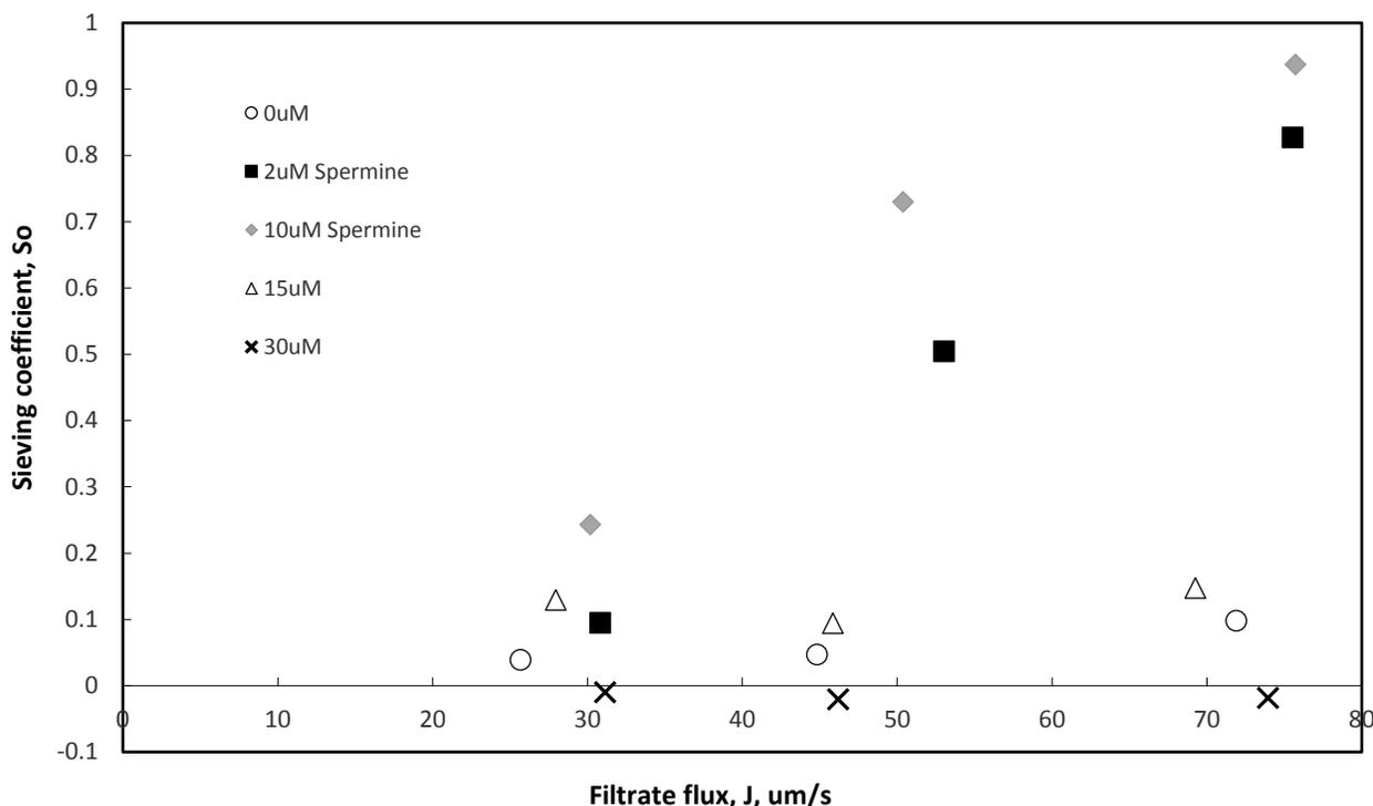
**Figure 3.** Sieving coefficient as a function of filtration for supercoiled isoforms in 10 mM NaCl TE buffer with different spermine concentrations.
