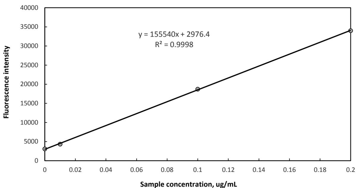
**Figure 2.** Calibration curve for determining DNA concentration from fluorescence assay.
