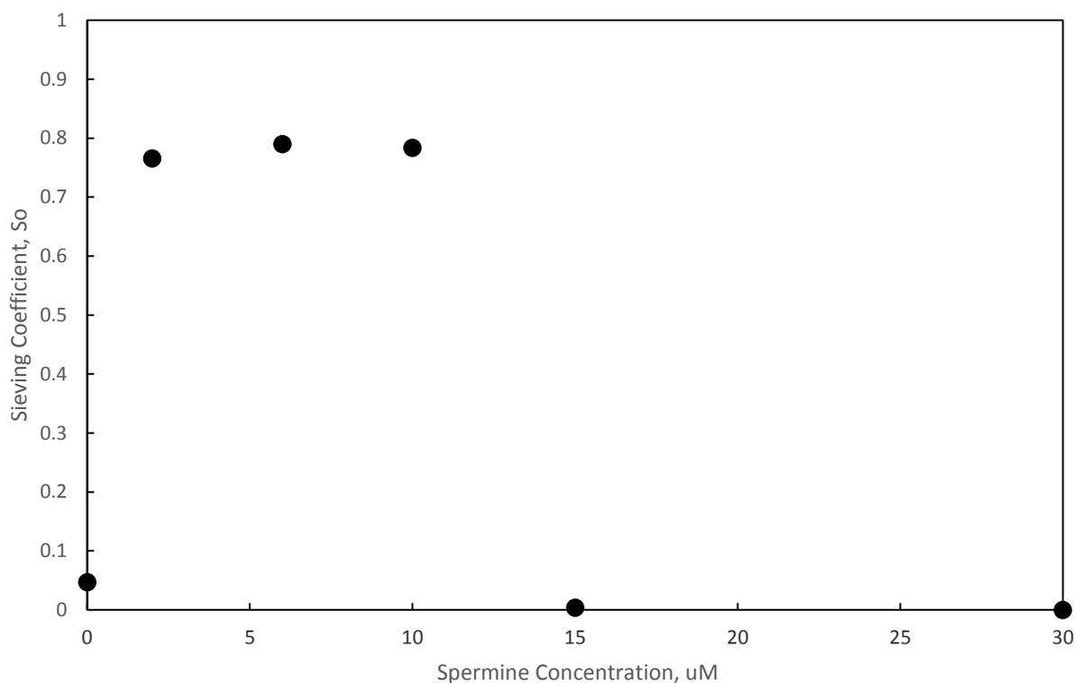
**Figure 4.** Sieving coefficient as a function of spermine concentration at a filtrate flux of  $50 \mu\text{m/s}$ .
