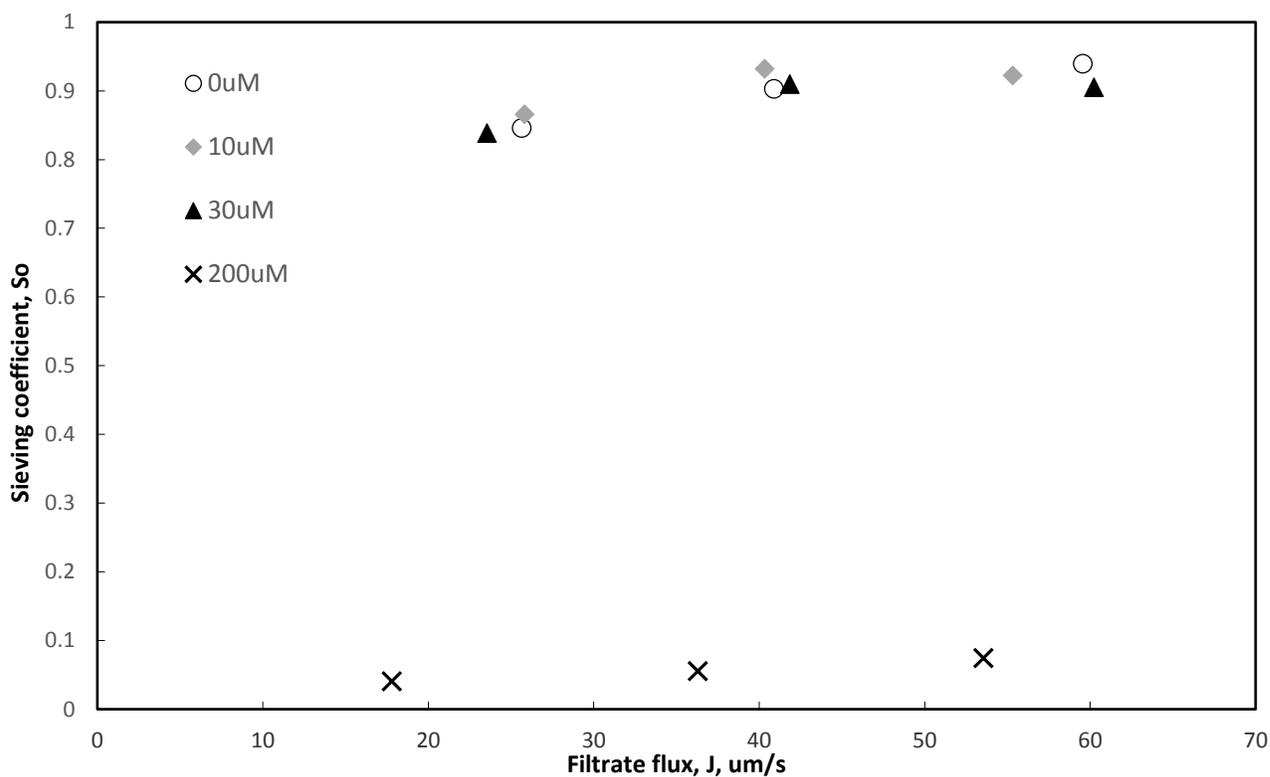
**Figure 8.** Sieving coefficient for supercoiled plasmid in 100 mM NaCl TE buffer.
