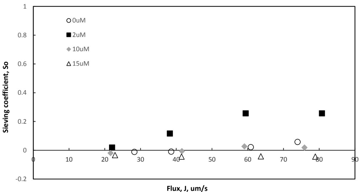
**Figure 12.** Sieving coefficient of the supercoiled MDY plasmid in 10 mM NaCl TE buffer through the Ultracel 300 kDa membrane at different spermine concentrations.
