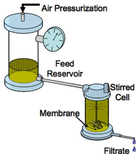
**Figure 1.** Diagram of stirred cell experiment set-up [13].
