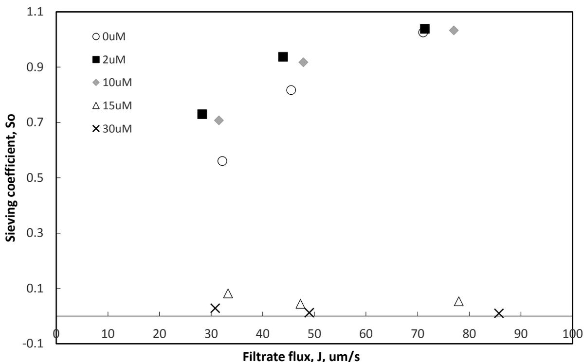
**Figure 5.** Sieving coefficient for linear plasmids as a function of the filtration flux in 10 mM NaCl TE buffer with different concentrations of spermine.
