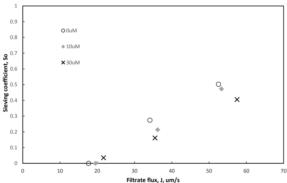
**Figure 7.** Sieving coefficient for open-circular plasmid in 100 mM NaCl TE buffer as a function of filtrate flux at different spermine concentrations.
