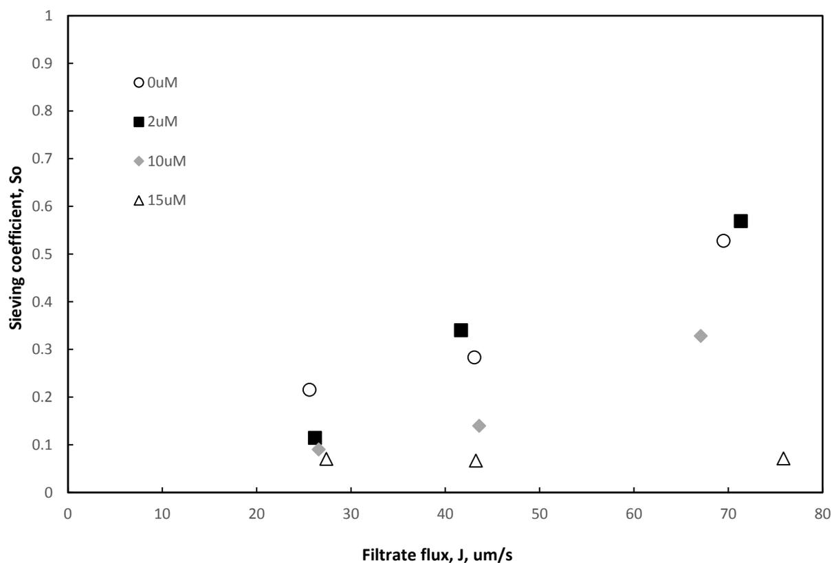
**Figure 11.** Sieving coefficient of supercoiled FDY plasmid in 10 mM NaCl TE buffer.
