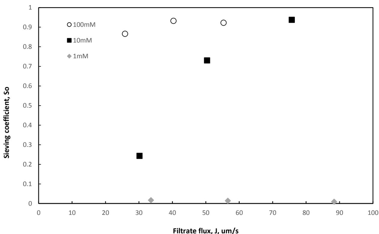
**Figure 9.** Sieving coefficient for supercoiled plasmids in 10  $\mu\text{M}$  spermine using 1, 10, and 100 mM NaCl in TE buffer.
