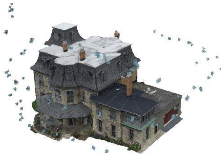
Figure 1: An example of photogrammetry using aerial photography. The blue points are camera locations.
