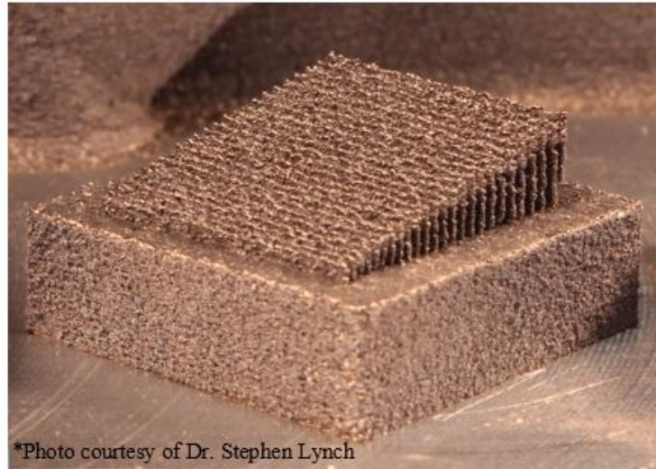
Figure 7: A pad with thin rectangular fins after fabrication using PBF.
