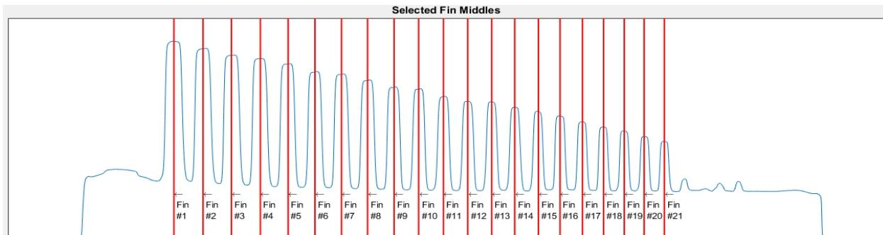
Figure 18: MATLAB returned side-view rendering of fins selected by the user for porosity analysis.
