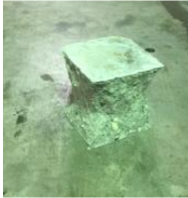
Figure 6: Typical Mortar Specimen after Failure
