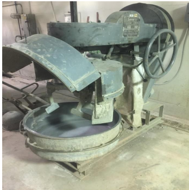
Figure 2: Photograph of pan mixer used for concrete mixing (Civil Infrastructure Testing and Evaluation Center, The Pennsylvania State University)
