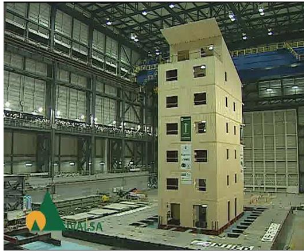
Figure 6-4. Seismic Testing at the Shaking Table Facility in Miki, Japan (Wind & Seismic, 2016)
