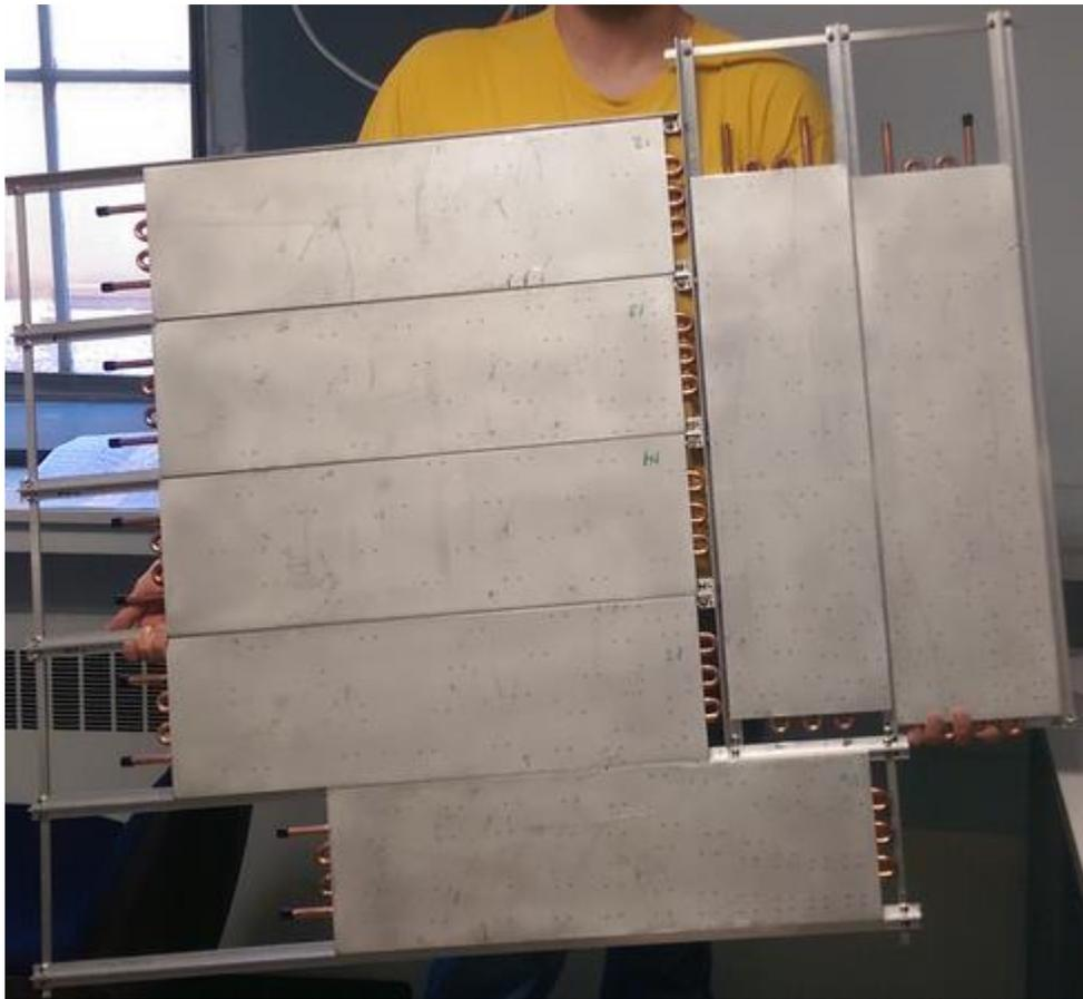
Figure 14- Cooling panels on aluminum frame before LEDs are attached.
