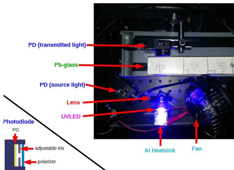
Figure 5-Schematic of LED wavelength optimization setup (top) with an image of the actual setup (bottom).
