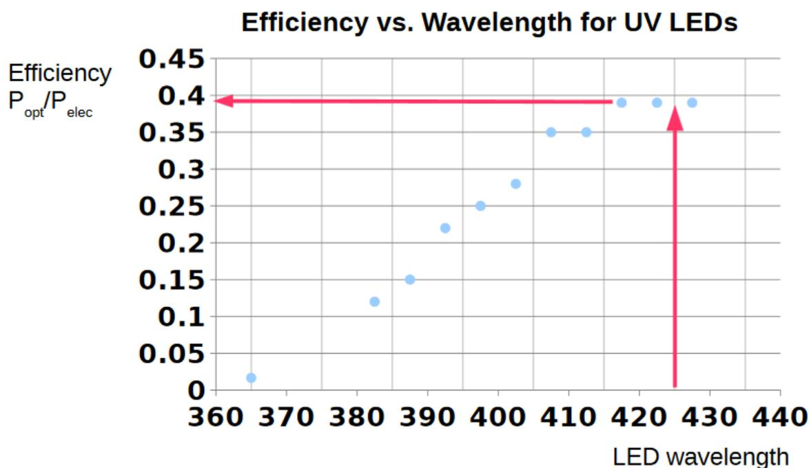
Figure 7- Efficiency vs Wavelength for different LEDs.
