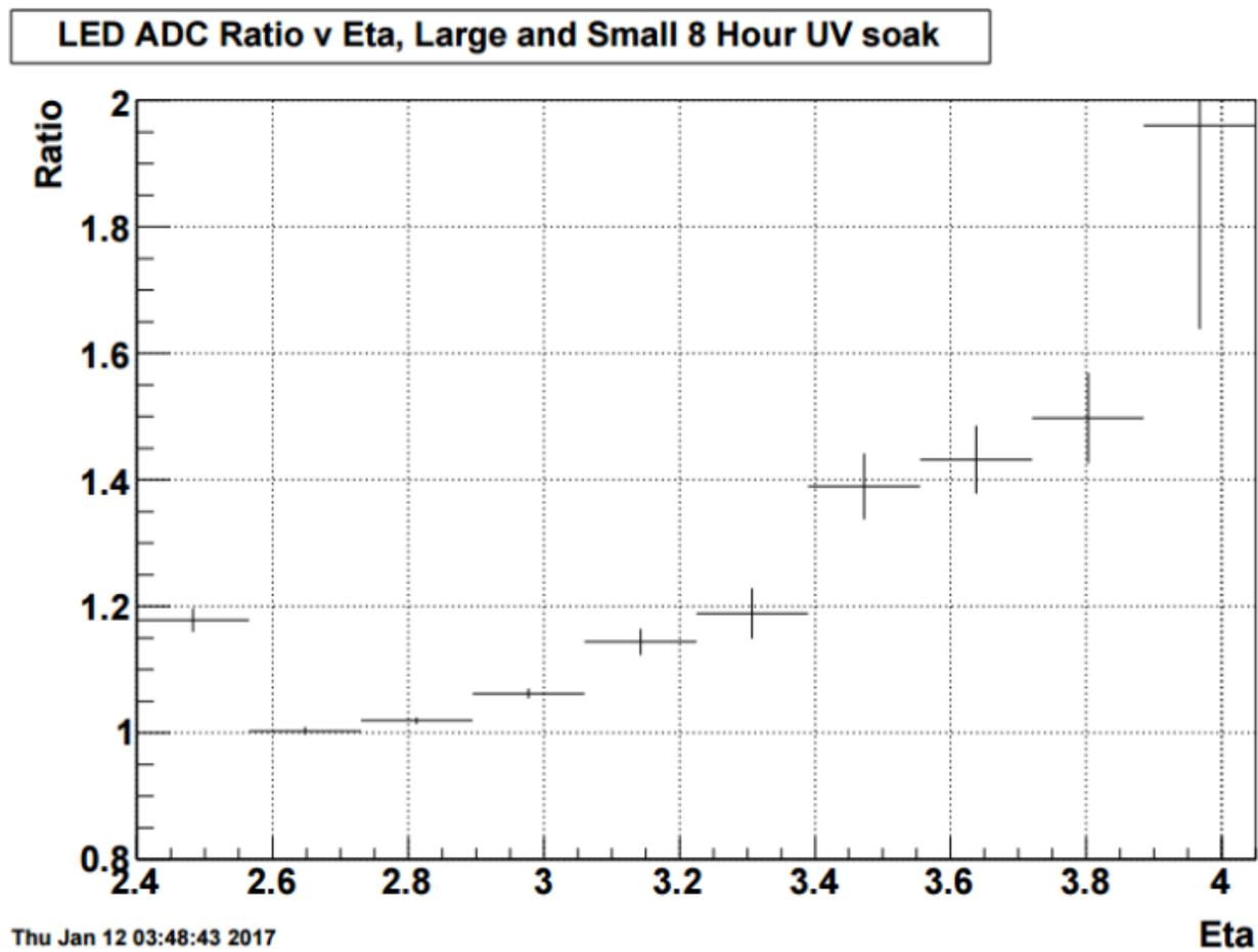
Figure 18- LED ADC ratio before and after an initial 8 hour UV soak vs Eta.
