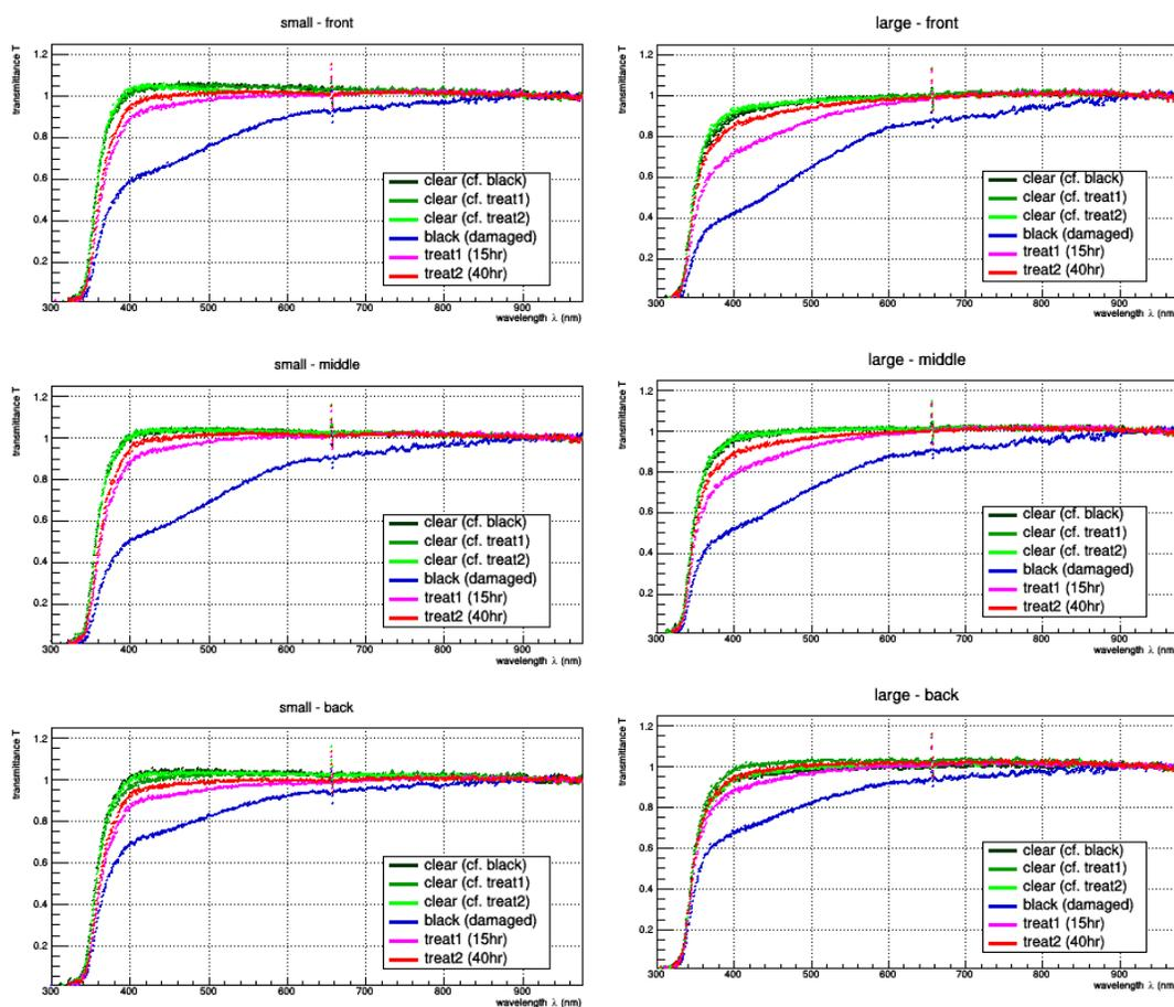
Figure 3-ADC count transmitted transversely through the cells at the front, middle, and back for small (left) and large (right) cells as a function of wavelength and time under a UV soak from the UVLED array.
