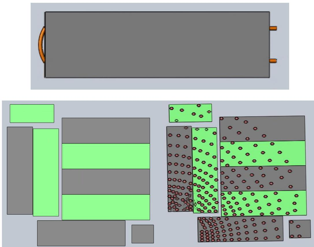
Figure 12- Solidworks models of the liquid cooling plate (top), plate placement for one quadrant of the detector (bottom left), and LED placement on the plates for one quadrant (bottom right).
