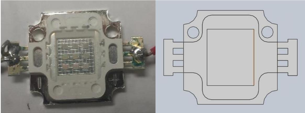
Figure 11- Image of the LED used (left) and Solidworks model of the LED (right).
