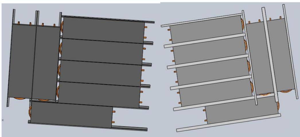
Figure 13- Frame with Cooling Panels SolidWorks Model.
