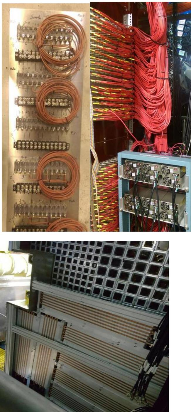
**Figure 16- Fuse blocks prepared (top left). The source and drain wires to the LED chains (top right). One quadrant of panels in place in front of detector (bottom).**
