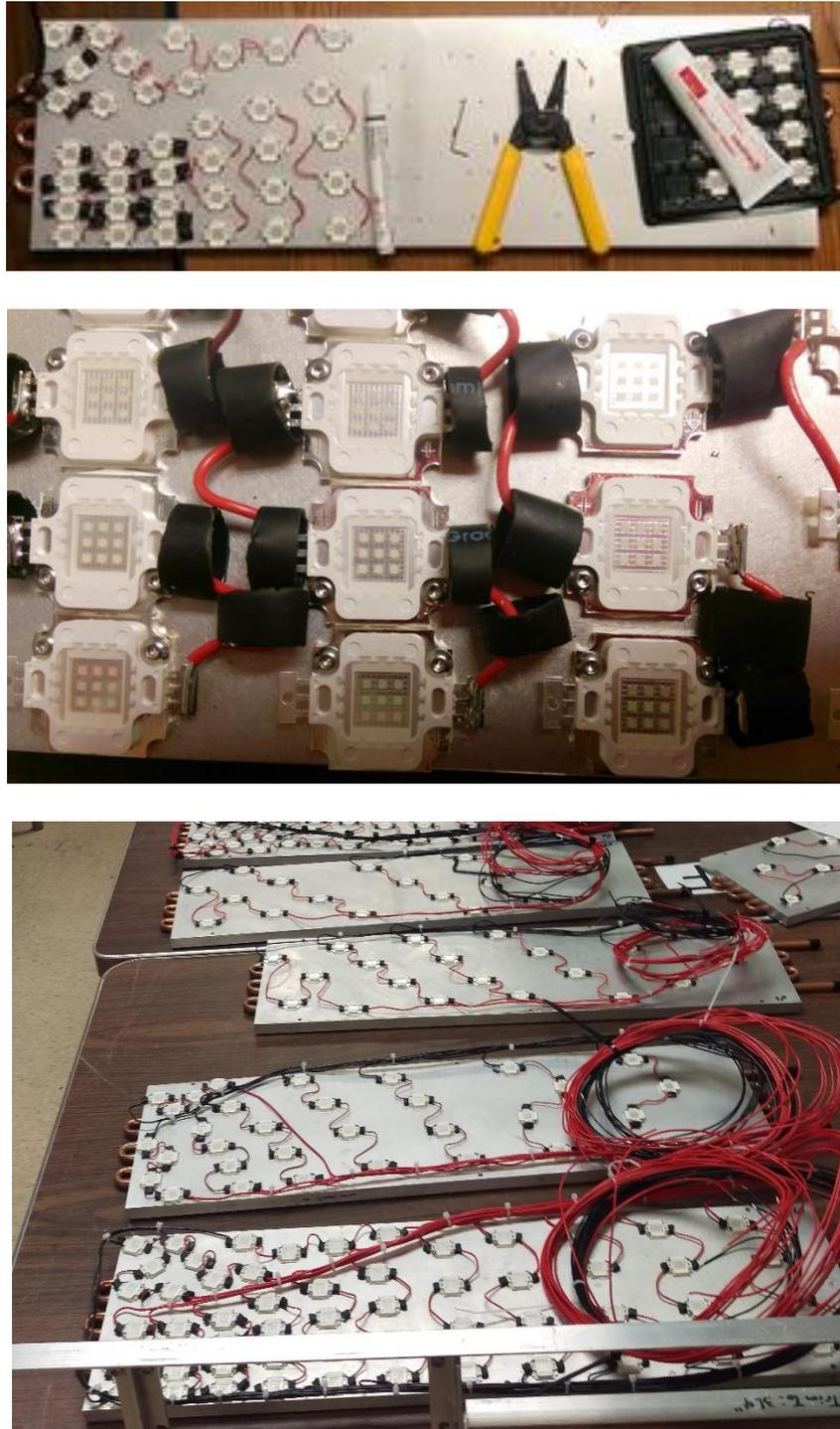
**Figure 15-Construction of liquid cooling panels. Top is panel in progress. Middle is a close up view of the heat shrink-wrap. Bottom is a few finished plates.**
