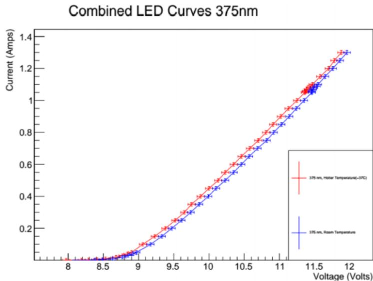
Figure 8- Current vs voltage curve for 375 nm LED. The linear relationship means the LEDs are ohmic.
