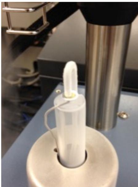
**Figure 8. The EG-water mixture is inside the DSC pan on the sample stage with the thermocouple next to the pan. (The mixture is yellow in this picture due to the presence of a small amount of the  $[\text{Ru}(\text{bpy})_3]^{2+}$  luminescent probe for other applications).**
