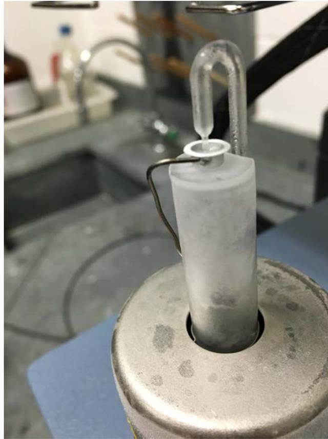
**Figure 22. Lengthening the tip of a penetration probe ensures its consistent and full penetration through the sample so the viscosity is more accurately reflected in the penetration rate.**
