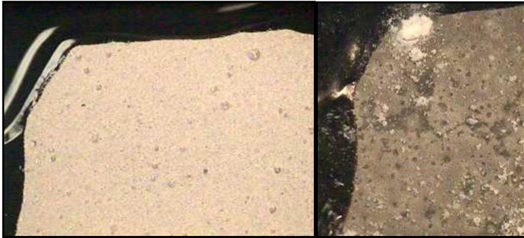
Figure 13. Surface images of Thk1w before testing (left) and after immersion and testing in HBSS (right).
