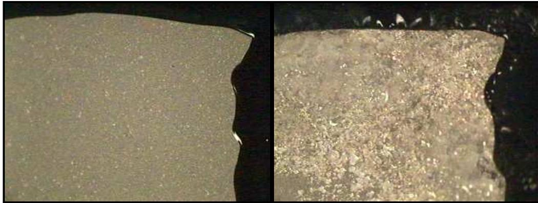
Figure 11. Surface images of Mg 87w before testing (left) and after immersion and testing in HBSS (right).
