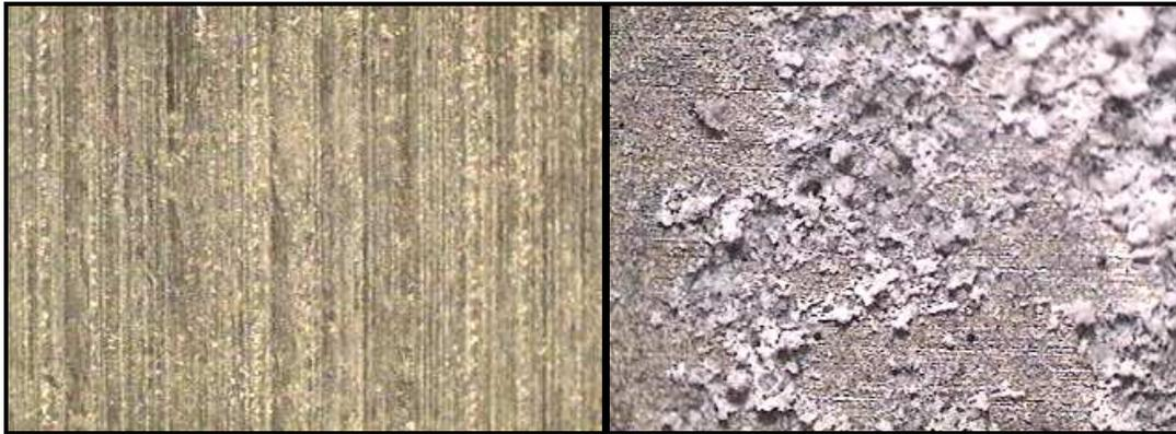
Figure 10. Surface images of AZ61 before testing (left) and after 28 days of immersion and testing in HBSS (right).
