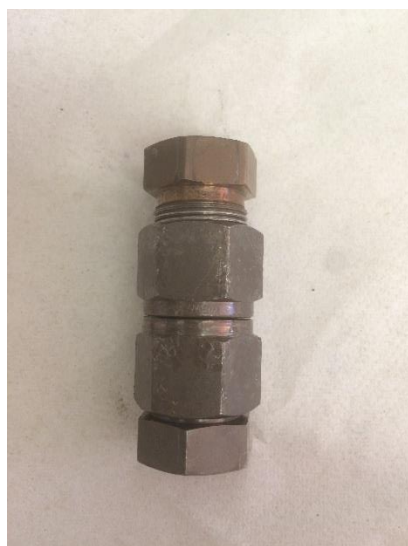
Figure 2 Swagelok Port Connector Reactor. The permanent end of the reactor is located at the bottom of the image, with the removable end at the top.
