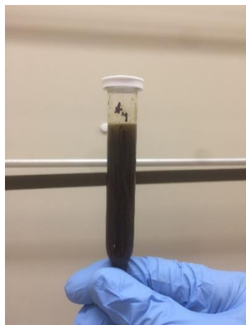
Figure 4 The crude product immediately following extraction. The extract is very murky and further work-up must be done before the three phases of the extract become visible.
