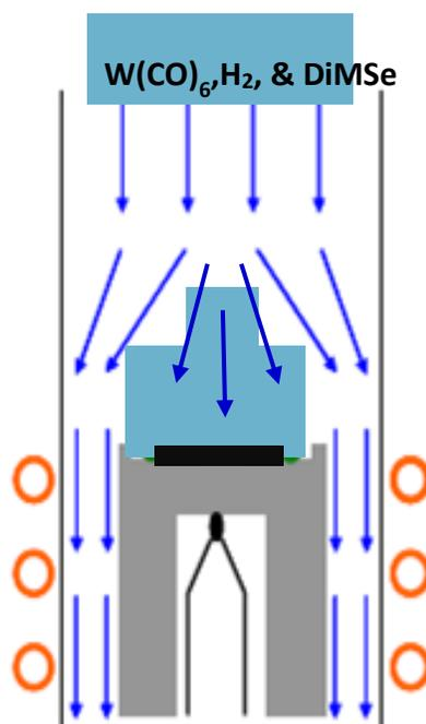
**Figure 9:** A general schematic of the reaction chamber, showing the hydrogen gas carrying the two precursors over the heated crucible/substrate where they deposit to form monolayered WSe<sub>2</sub>.
