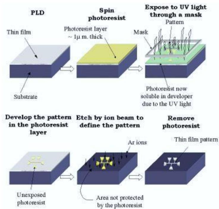
**Figure 7** : General schematic of the photoresist lithography process utilized to leave the growth inhibiting polymer layer in desired regions. Note that this schematic does not show the reactive ion etching or plasma steps involved.
