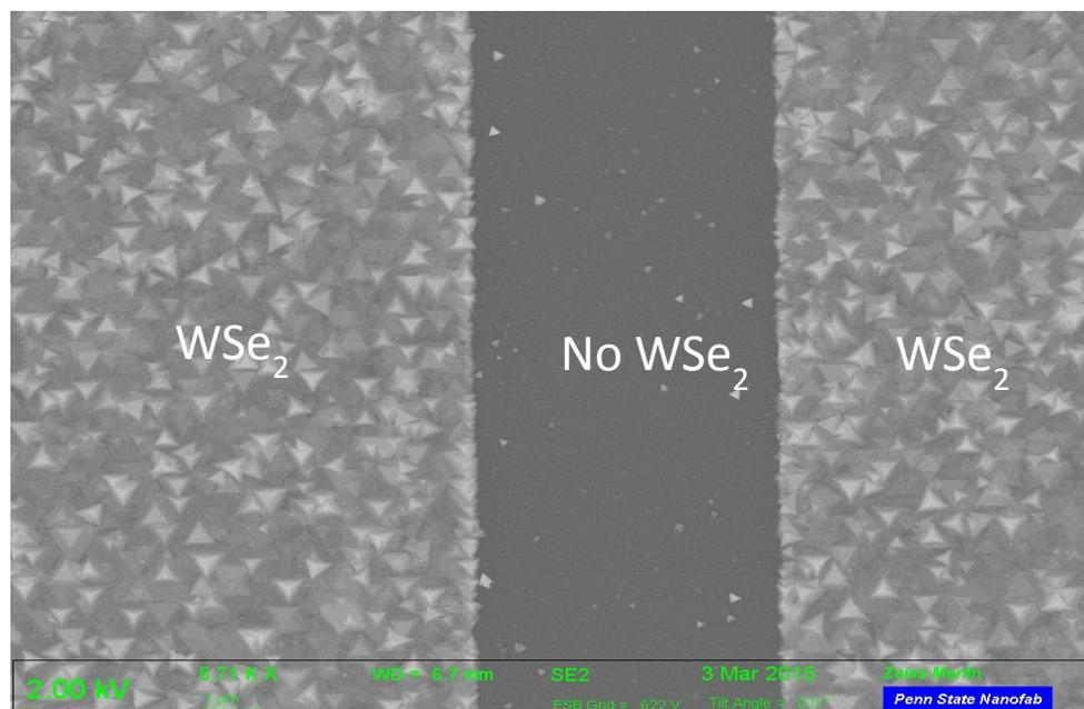
**Figure 13 (previous page):** SEM image of boundary between growth (non-functionalized) and inhibition (functionalized) region
