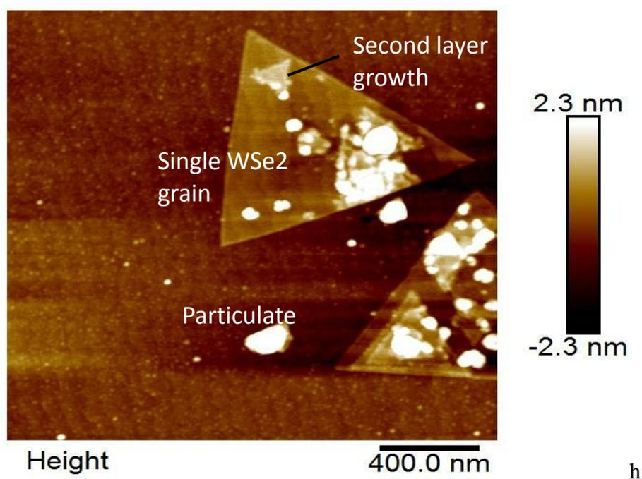
**Figure 11:** AFM image close up of the individual triangular  $\text{WSe}_2$  grains on sapphire substrate. The high elevation (white) dots are random particulates on the surface.
