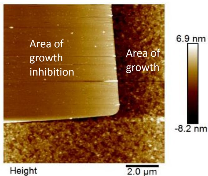
**Figure 10:** AFM image of WSe<sub>2</sub> (the small triangular grains) on a sapphire substrate. Note the clear definition between the clear area of growth inhibition and that of growth.
