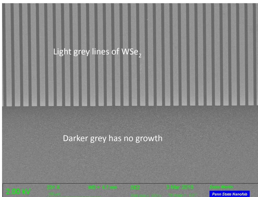
**Figure 12 (previous page):** SEM image of a selective growth sample. The lighter grey lines indicate areas of growth, while the darker lines show areas of inhibition.
