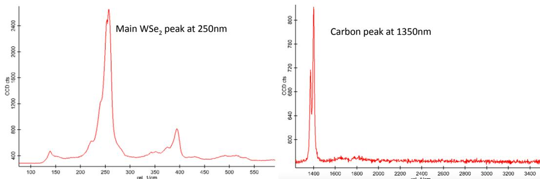
**Figure 14:** (Left) Shows a Raman spectrum of a sample. Notice the main WSe<sub>2</sub> peak located at around  $\sim 260 \text{ cm}^{-1}$ . (Right) Shows a Raman spectrum of a region of inhibition. The peak at 1350nm is an indicator of the carbon-based polymer residual layer
