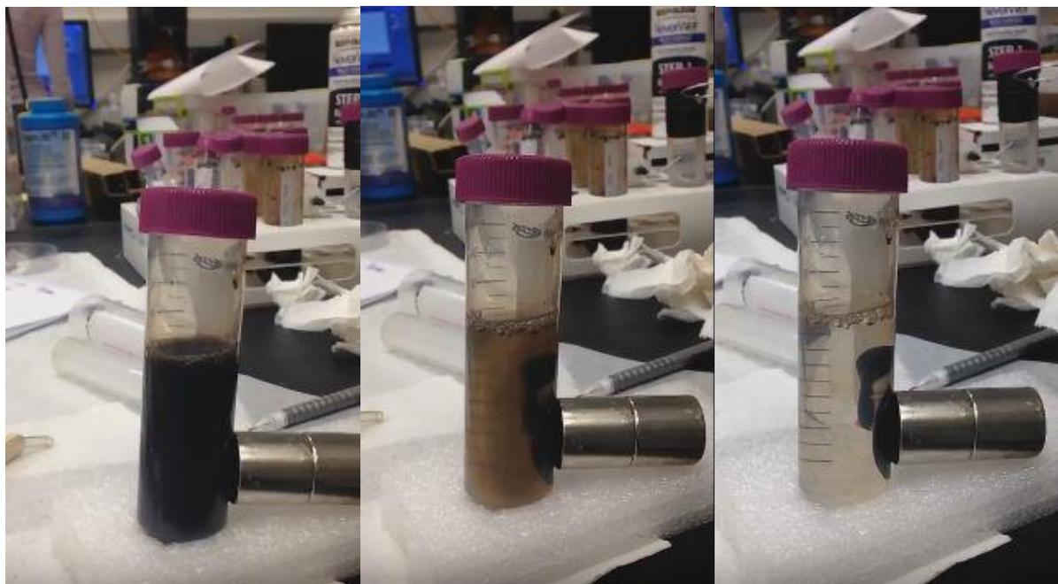
**Figure 3 Soluble and Magnetic Properties of Synthesized Nanoparticles**
