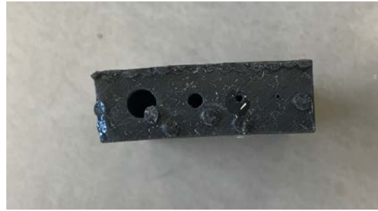
Figure 6: Resin Leakage after Vacuum
