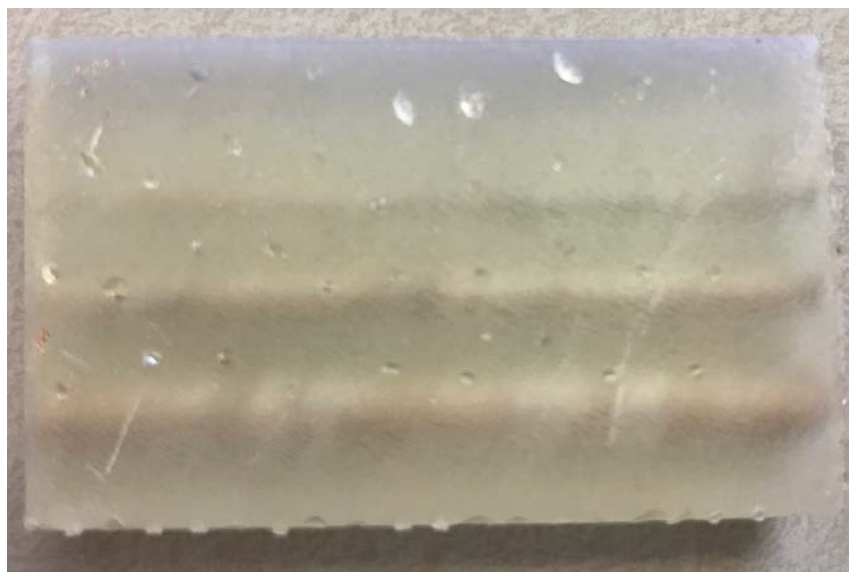
Figure 8: Conductivity Test Block. Hole Diameter from top to bottom: 0.5 mm (closed off with resin), 1 mm, 2 mm, and 4 mm.
