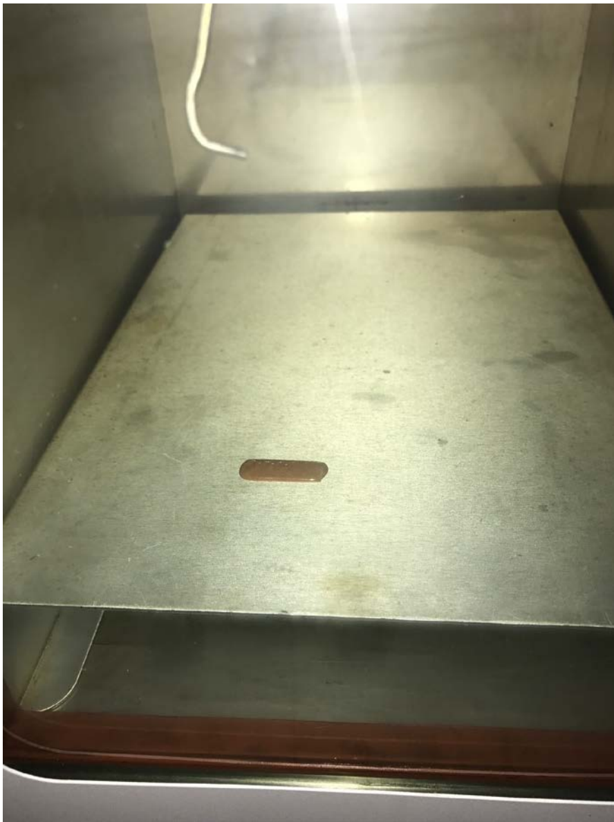
Figure 3: Melted Virtual Foundry Filament in Oven
