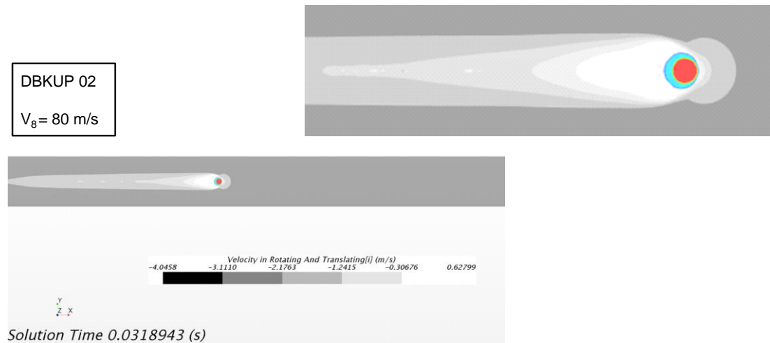
Figure 12: View of 473 \mu\text{m} Droplet Near the Start of Simulation Approaching DBKUP 02 Section
