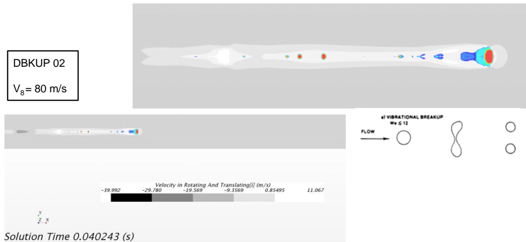
Figure 13: Onset of Vibrational Breakup (473 \mu\text{m} Droplet, DBKUP 02 Section) – Breakup Mechanism Image Taken from Pilch and Erdman 10
