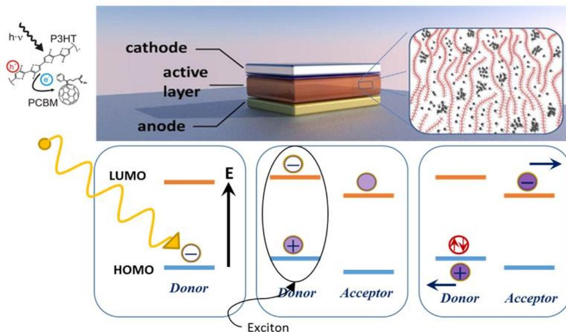
**Figure 1. Diagram showing the beginning process of electricity generation system in an organic solar cell with p-type donor P3HT and n-type acceptor PCBM. The major steps, excitation, dissociation, and charge separation are visualized.**
