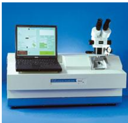
Figure 3-3 Fischione Low Angle Ion Mill model 1010 used to prepare samples for OIM.
