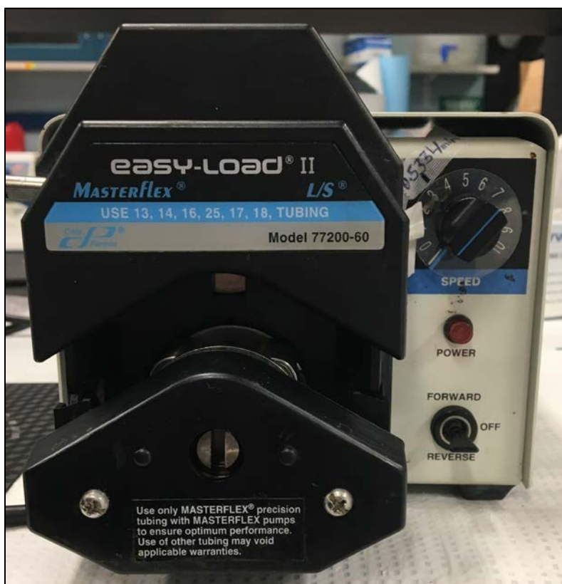
Figure 14: Control panel of peristaltic pump. Flow rate is set using an unlabeled knob.
