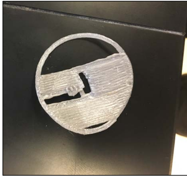
Figure 25: 3D printed gasket with 1 mm/s printing speed. Print was aborted after excessive filament size and low resolution were observed.
