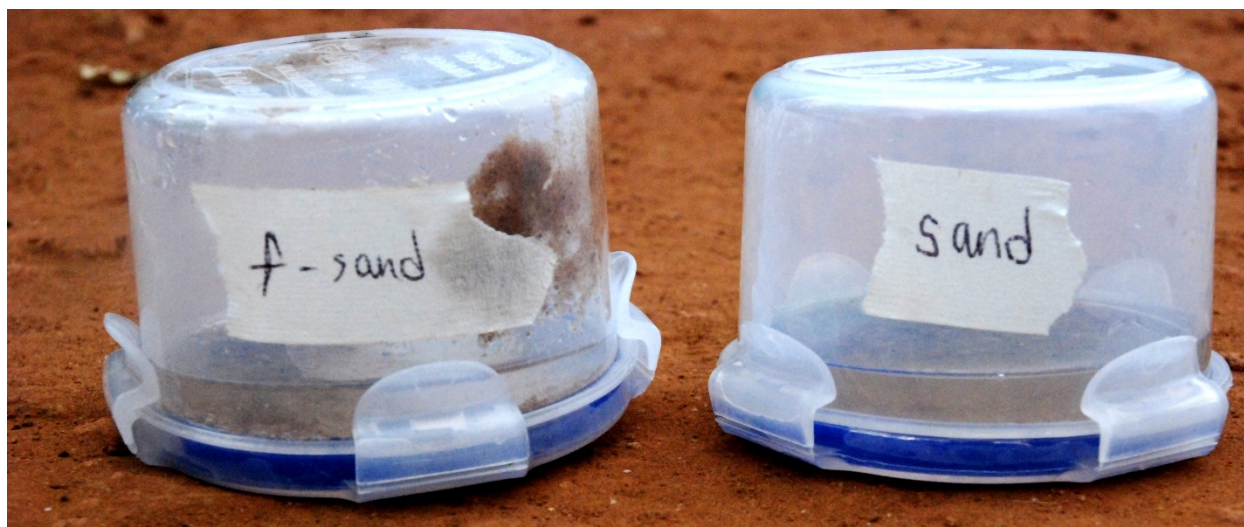
Figure 16: Moringa-coated-sand from made in the field in Rwanda with seed cake waste product, rainwater, and natural sand found outside, passing the “stick” test.
