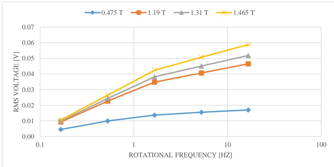
**Figure 14: RMS voltage per winding at varying magnet grade over a range of discrete rotational velocities. As the thickness of the magnet increases, the RMS voltage output increases. As the grade of the magnet increases, the RMS voltage output increases.**
