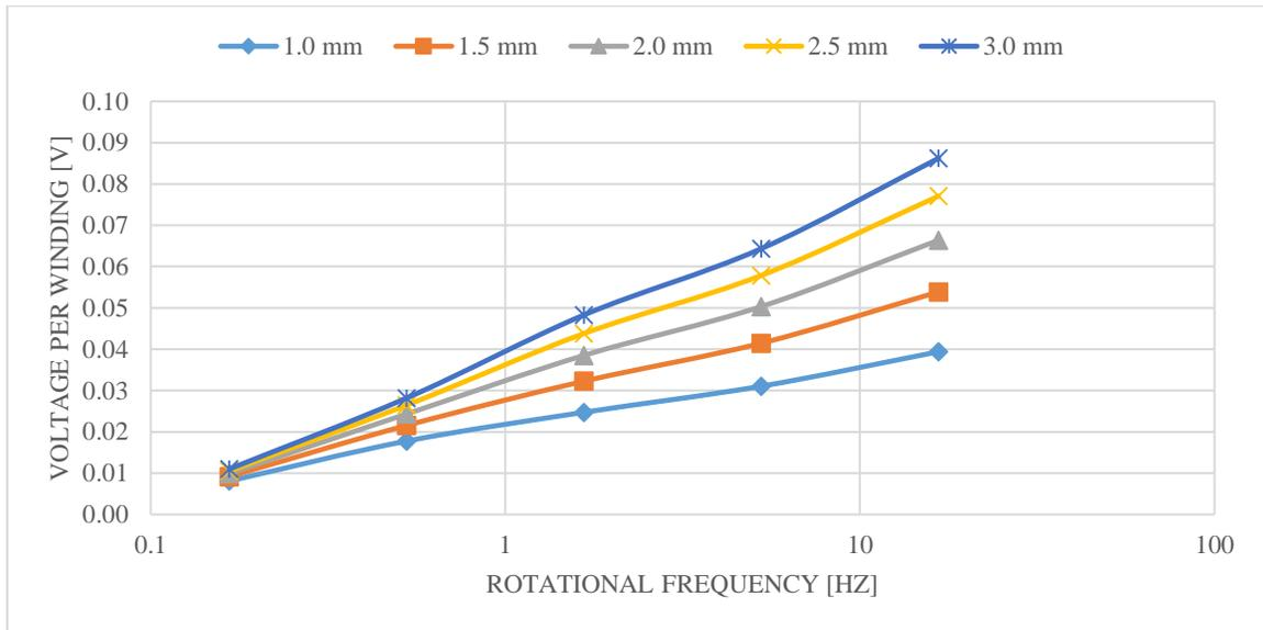
**Figure 16: RMS voltage per winding at varying Halbach array thickness over a range of discrete rotational velocities. As the thickness of the Halbach array increases, the RMS voltage output increases.**
