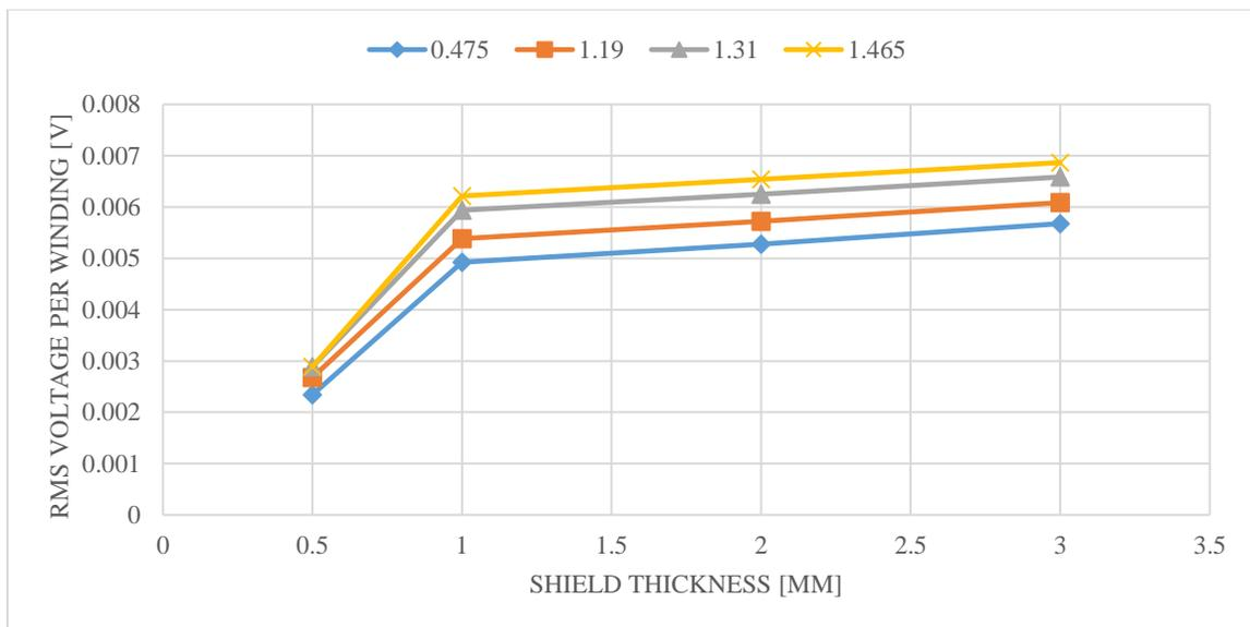
**Figure 20: RMS voltage of an alternator at 10 Hz for varying shield thickness and permanent magnet grade**
