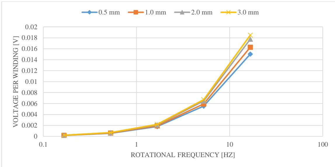
**Figure 17: RMS voltage per winding at varying shield thickness over a range of discrete rotational velocities. As the grade of the shield thickness increases, the RMS voltage output increases.**
