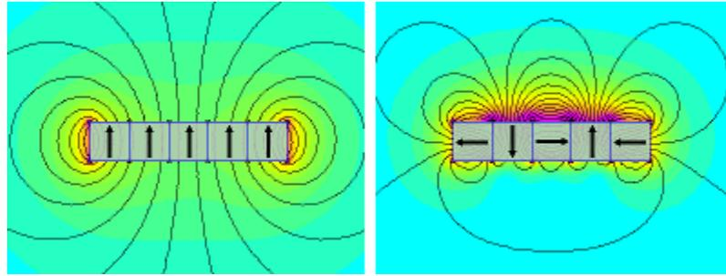
**Figure 3: Standard magnetic array (left) compared to a Halbach array (right). Note the concentration of magnetic flux at the top surface. (K&J Magnetics, n.d.)**
