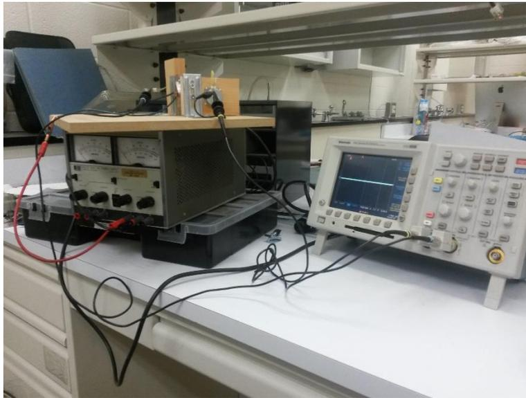
**Figure 8: Example setup, including generator, DC power supply, and oscilloscope.**
