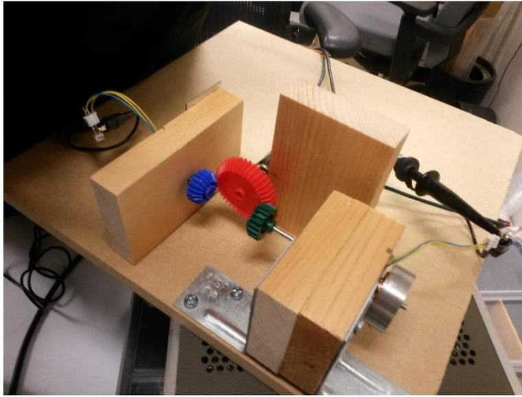
**Figure 7: Alternator-motor connections. The large red gear is connected to the motor, and provides power to the alternators (the small green and blue gears).**
