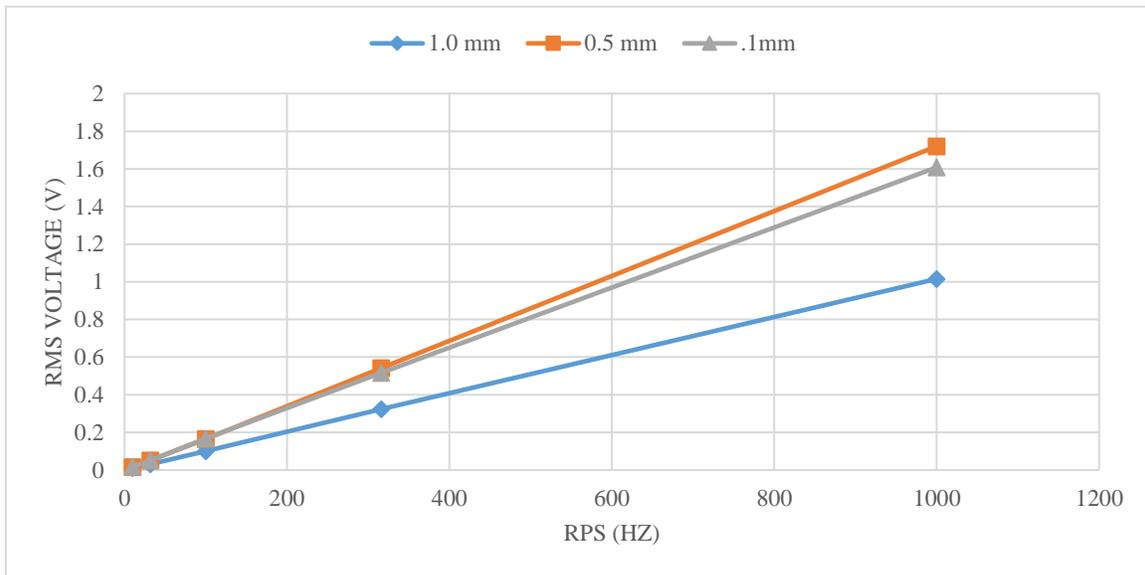
**Figure 21: RMS voltage versus shaft frequencies for various magnet-core gap widths. The two smallest gap sizes present little change, but the largest gap shows a great decrease in voltage output.**
