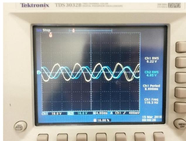
**Figure 9: Typical output from the larger motor. The Channel 1 voltage, channel 2 voltage, and period are shown to the right of the voltage-time plot.**
