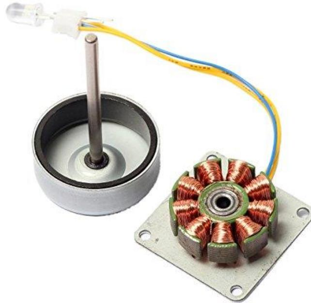
**Figure 4: CrocSee 3-phase alternator, image provided by CrocSee at [www.amazon.com](http://www.amazon.com).**
