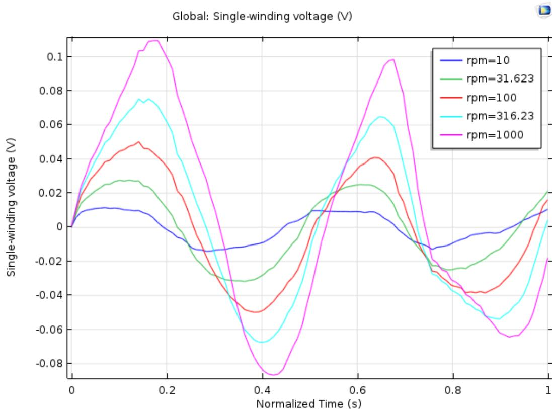
**Figure 6: Example COMSOL output graph - Voltage over a single phase in a three-phase alternator winding for five distinct rotational velocities. Note that the amplitude of the semi sinusoidal wave increases with velocity, which is expected.**
