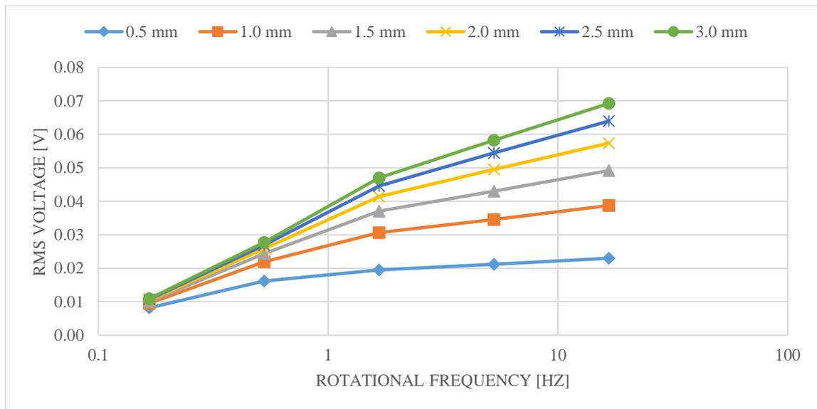
**Figure 13: RMS voltage per winding at varying magnet thicknesses over a range of discrete rotational velocities. As the thickness of the magnet increases, the RMS voltage output increases.**
