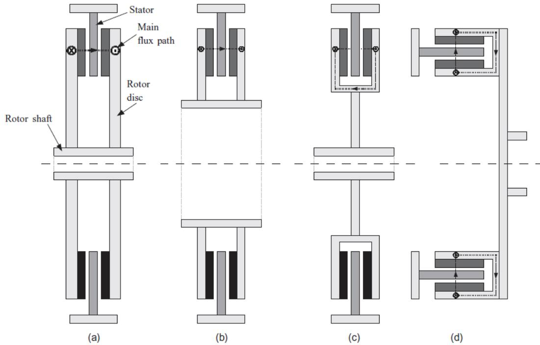
**Figure 1: Cross section of double-sided axial-flux machine (Mueller & McDonald, 2009). (a) Baseline design (b) Increasing rotor shaft radius means the thickness of the rotor discs can be reduced (c) 'C' core machine with extra flux path (d) Radial-flux 'C' core**
