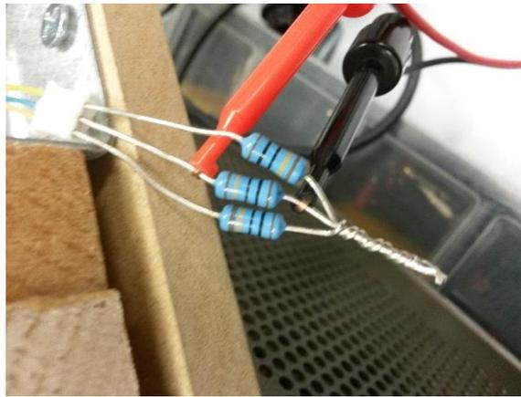
**Figure 11: Resistor and probe wye configuration to measure voltage drop across resistor.**
