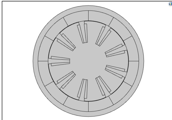
**Figure 5: 2-D generator model for initial analysis. This model is based upon the commercially available generator with magnets of increased thickness**
