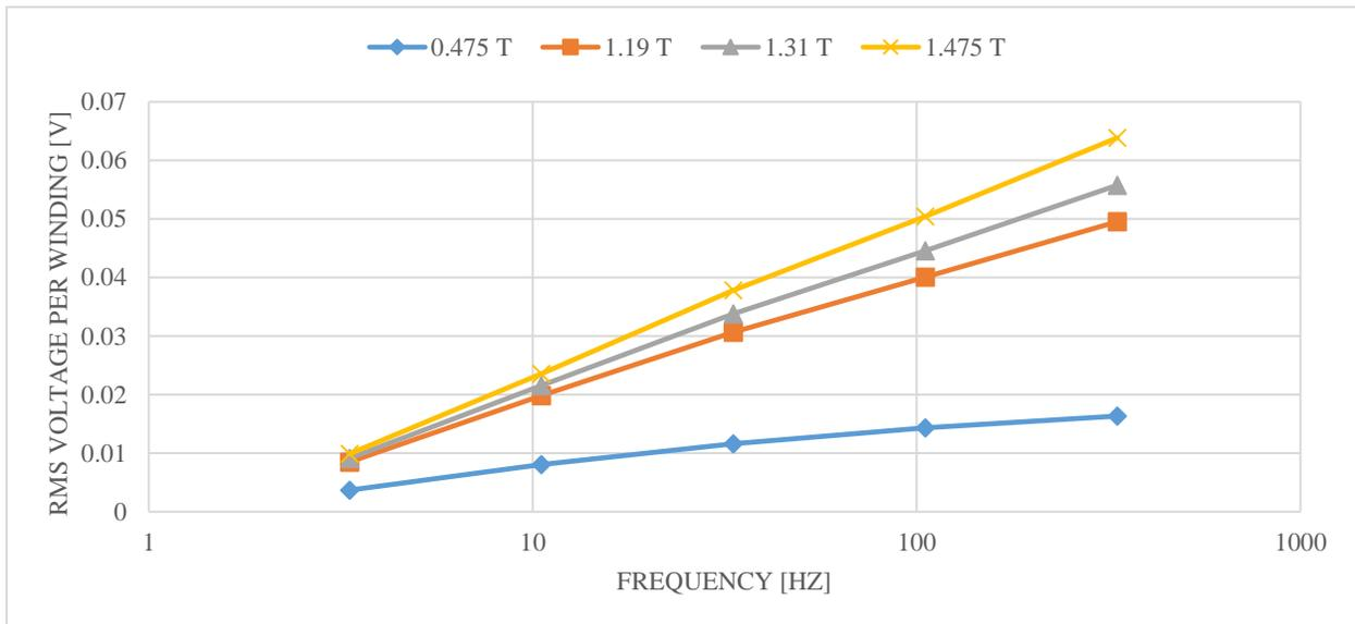
**Figure 15: RMS voltage per winding at varying Halbach array grade over a range of discrete rotational velocities. As the thickness of the magnet increases, the RMS voltage output increases. As the grade of the Halbach array increases, the RMS voltage output increases.**
