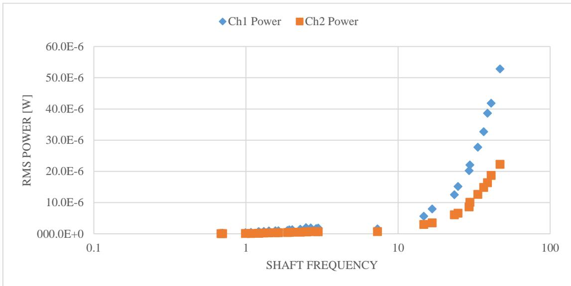
**Figure 19: RMS power output of stock alternator and prototype. The power values within the graph are calculated from the voltage data.**
