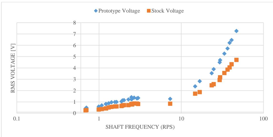
**Figure 18: Experimental output of modified vs. stock alternator. Specific data points are shown in each data series. The gap between 3 and 7 revolutions per minute is due to the velocity range differences between motors.**
