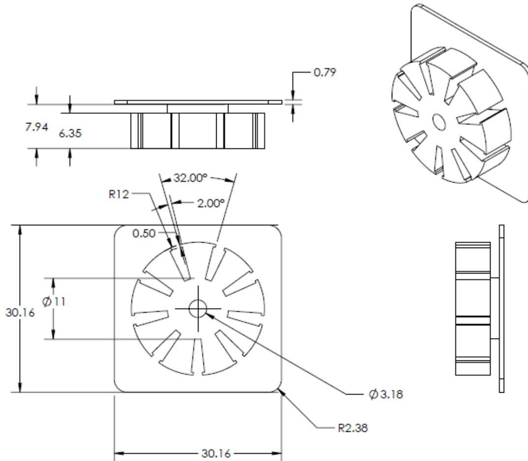
Stator and core dimensions
