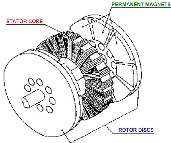
**Figure 2: Axial-flux permanent-magnet alternator (Caricchi, Crescimbin, Capponi, & Solero, 2001).**
