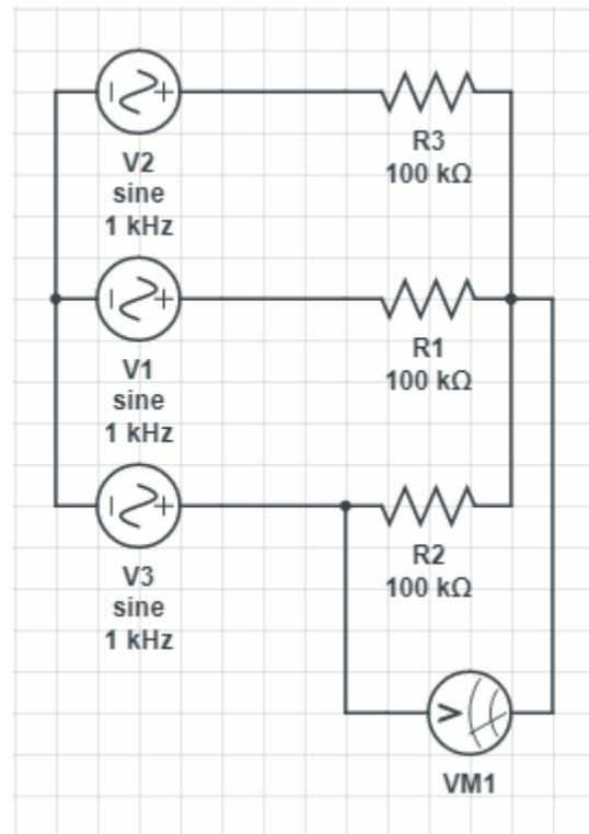
**Figure 12: Circuit diagram of single alternator test setup. Note that the voltmeter represents the oscilloscope and has a built-in ground. Circuit designed using [www.circuitlab.com](http://www.circuitlab.com).**
