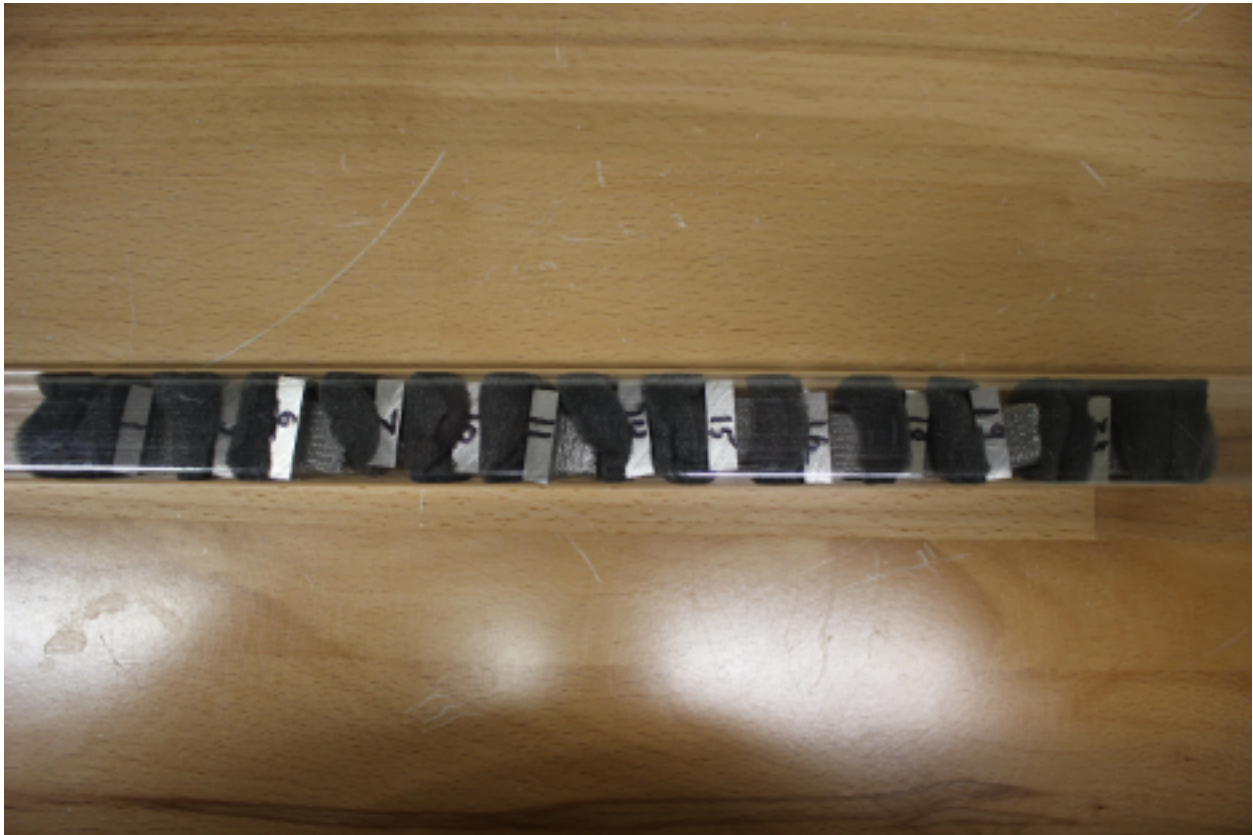
Figure 2.4: Cubes mounted in the plastic tube to be CT scanned.
