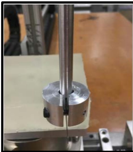
Figure 3 Experimental set up used in earlier scalpel compliant testing. A large clamp was used to secure scalpel blade. The large mass acted as a damper.
