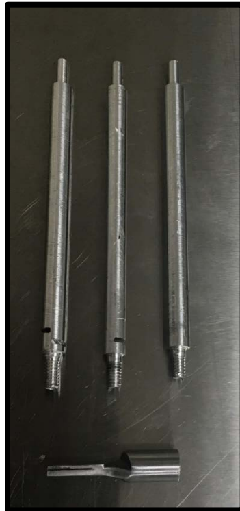
Figure 9 Final machined parts. Top left: double slit compliant geometry scalpel handle. Top middle: single slit compliant geometry scalpel handle. Top right: no compliant geometry scalpel handle. Bottom: Scalpel blade holder.
