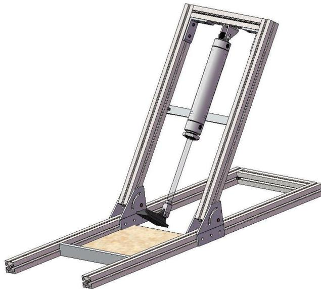
Figure 12 – SolidWorks model of proposed dynamic tester design. Note a comprehensive Bill of Materials is in the APPENDIX A.
