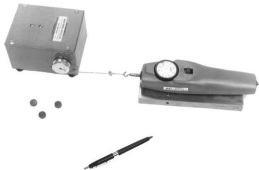
Figure 2 – Example of a Horizontal Pull Slipmeter (HPS), a drag-sled-type device.
