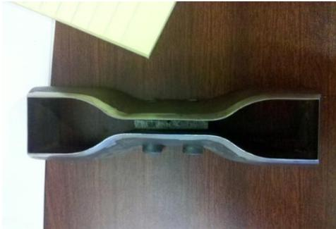
**Figure 21 – ASTM D412 Standard Tensile Bar Cutter** Was used in Generation 2 material testing in order to better produce tangible data.
