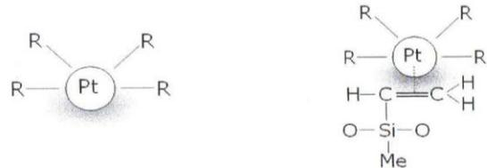
**Figure 2 - Platinum Cure Reaction** The platinum catalyst reacts with the double bond in the vinyl group, creating an active site for polymer chain propagation. Courtesy of Polymer Engineering Center, U of Wisconsin-Madison.
