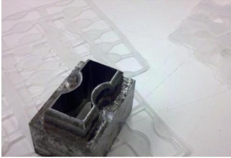
**Figure 20 – Non-Standard Tensile Bar Cutter** Was used in Generation 1 material testing.
