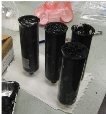
**Figure 4 – Cartridges After Loading** Shows Carbon Black charges loaded into feed system cartridges. Cartridges were placed in the retainer body and fed through the injection molding machine.
