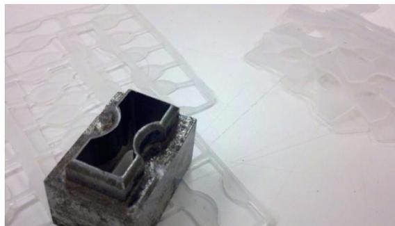
Figure 3 – Die Cutter and Samples Shows the die cutter used to make samples from plaques, as well as cut samples.
