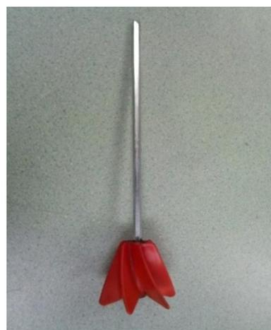
**Figure 19 – Paint Mixing Attachment for Power Drill Used in Generation 2 Mixing Methods** Shows the paint mixing attachment that was used to improve the mixing stage of the research project.
