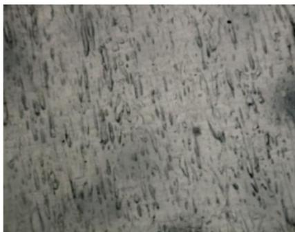
**Figure 31 – Filler Dispersion from Gen. 2 Mixing Methods** Shows the filler dispersion as seen in Generation 2 mixing.
