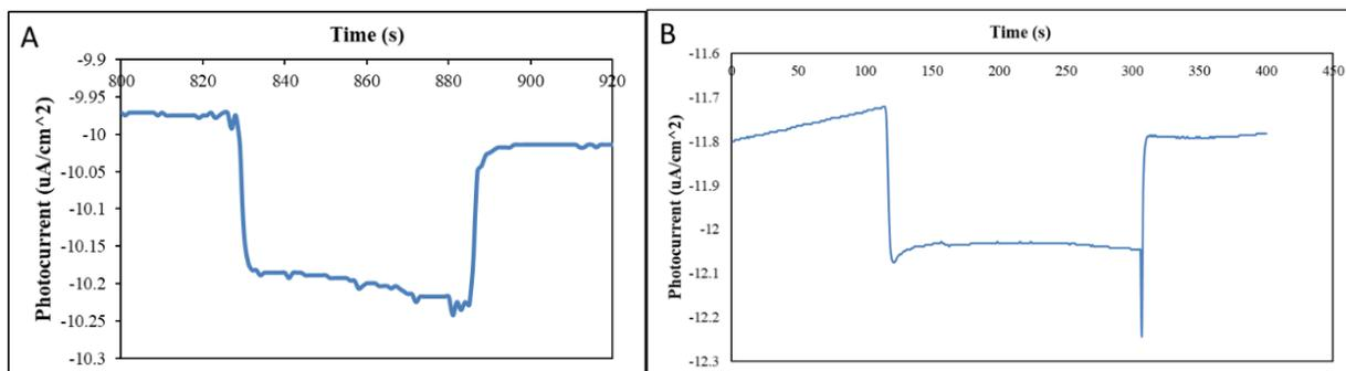
**Figure 13. Photocurrent profiles of PSI-BCP organic photovoltaic. A. On day 1 of testing. B. On day 35 of testing.**
