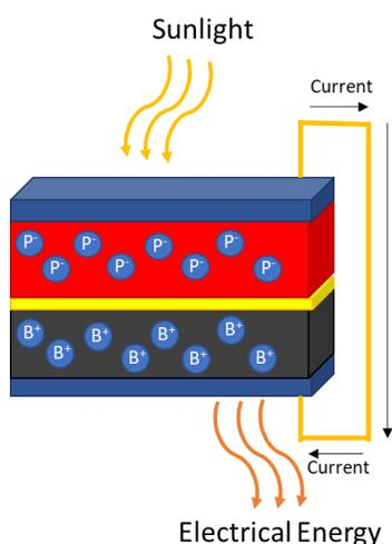
**Figure 1. Schematic of commercial solar panel. Doping with negatively charged phosphorus ions and positively charged boron ions promotes electron transfer from top to bottom upon introduction of sunlight to produce electrical energy.**
