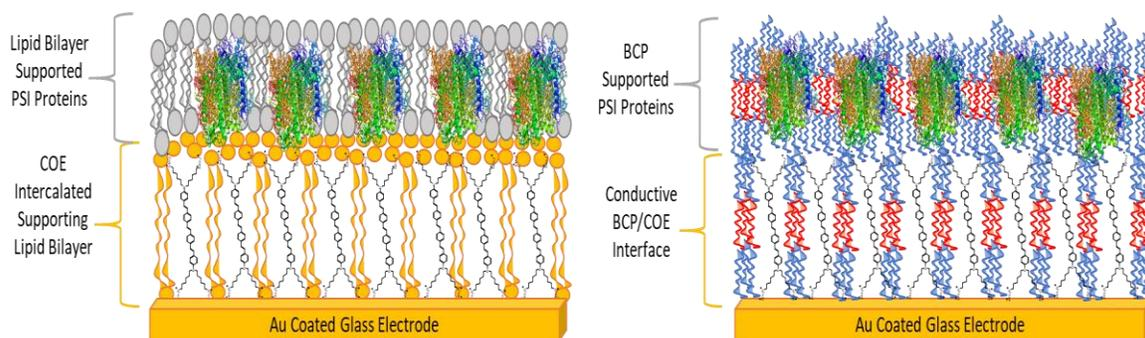
**Figure 2. Comparison of lipid bilayer supported photovoltaic to block copolymer photovoltaic system. The general bilayer supported protein structure is maintained in both systems.**
