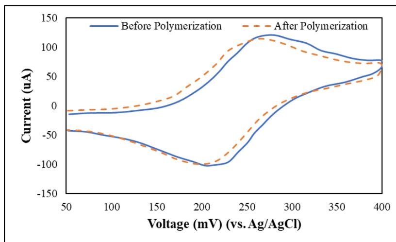
**Figure 16. BCP interface with COEs before and after UV polymerization.**
