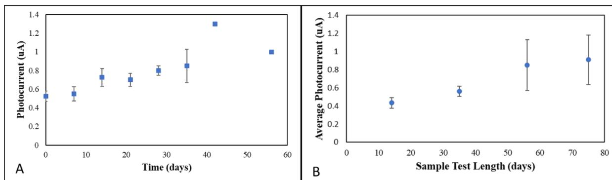
**Figure 12. Stability testing for PSI-BCP samples. A. Average photocurrent for each weekly testing period. B. Average photocurrent of each tested sample.**
