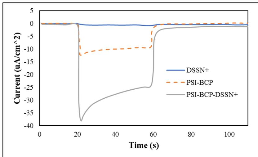
**Figure 11. Photocurrent measurements over 40 seconds for modified gold electrodes with and without PSI proteins.**
