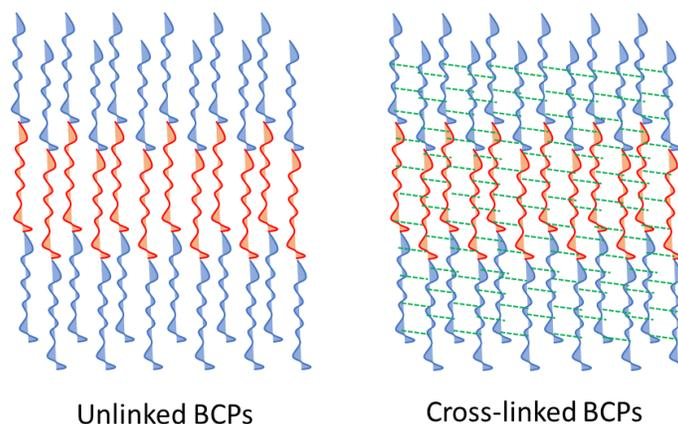
**Figure 6. Cross linking enhances the overall stability of BCP membrane systems.**
