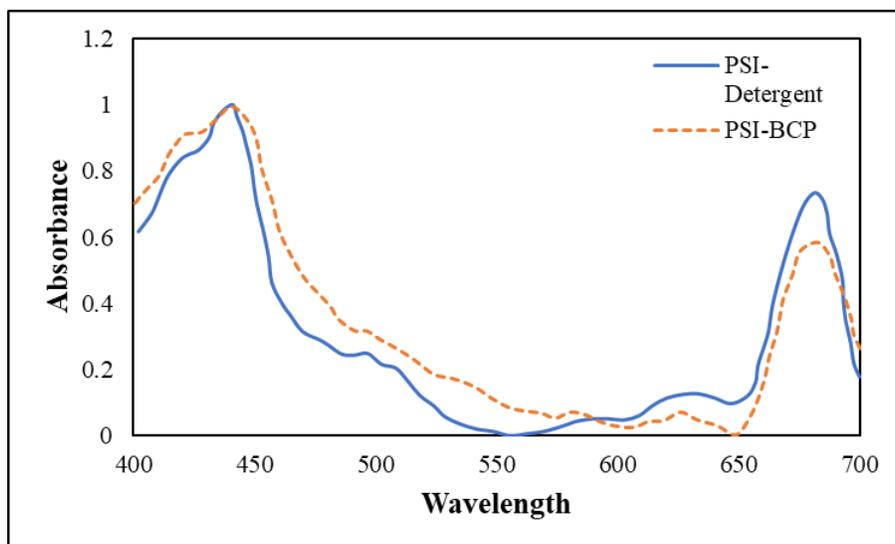
**Figure 14. UV-Vis spectra of PSI in detergent micelles or in a BCP membrane.**
