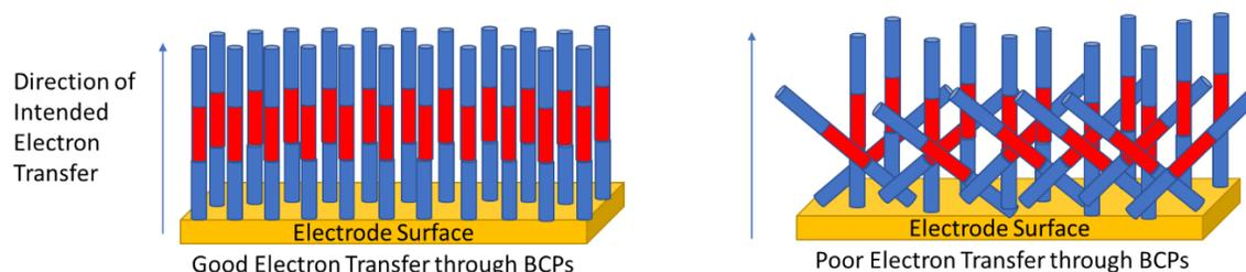
**Figure 4. Comparison of cylindrically arranged BCP units for electron transfer through a BCP COE-intercalated membrane. When BCPs and COEs are misaligned, electron transfer cannot occur efficiently because the paths for electron travel are not all direct and continuous from the electrode to the protein.**
