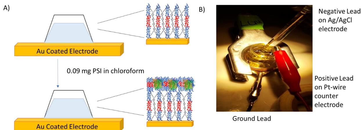
**Figure 9. PSI integration and photoelectrochemical testing. A. Procedure for integrating PSI proteins atop the BCP bilayer. B. Setup of electrochemical cell for single base potential voltammetry readings.**
