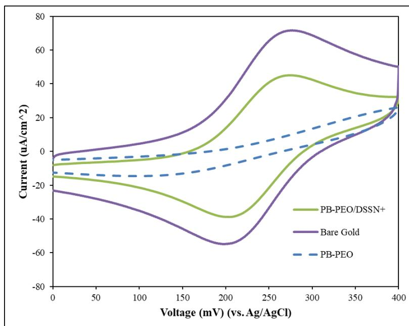
**Figure 10. Cyclic voltammetry of modified (PB-PEO/DSSN+ and PB-PEO) and unmodified (bare gold) electrodes.**
