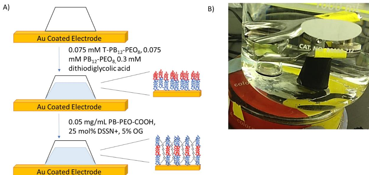
**Figure 8. Schematic of BCP self-assembled monolayer (SAM) procedure. A. Assembly of a SAM on a gold electrode. B. Dialysis procedure.**
