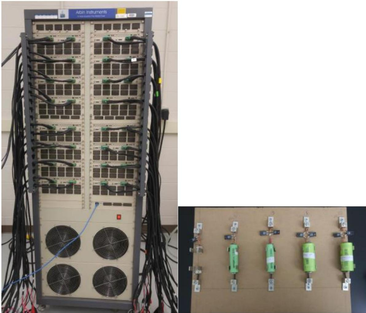
Figure 13. Left picture, the lab cycler used to apply input current profile on the batteries. Right picture, the battery setup with the resistor s in the battery validation process.
