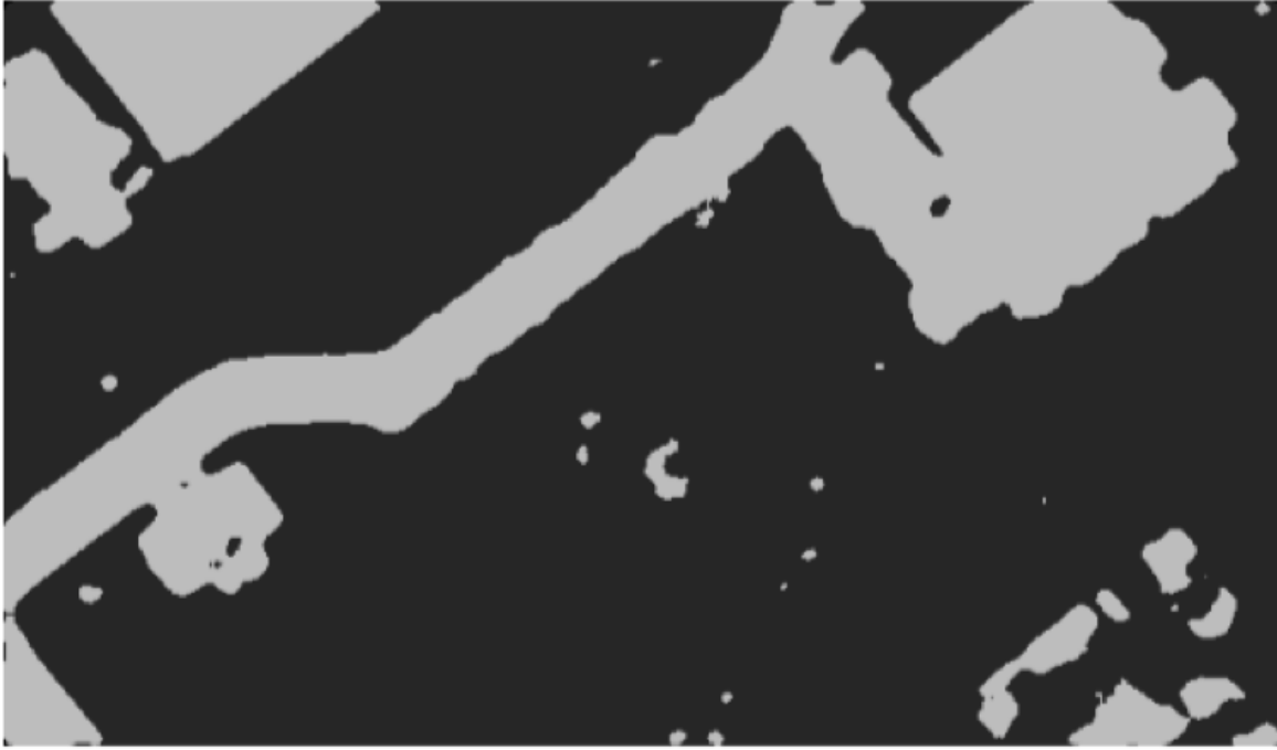
Figure 2.4: Resulting power map from applying k-means segmentation and 9x9 median filter. [10]
