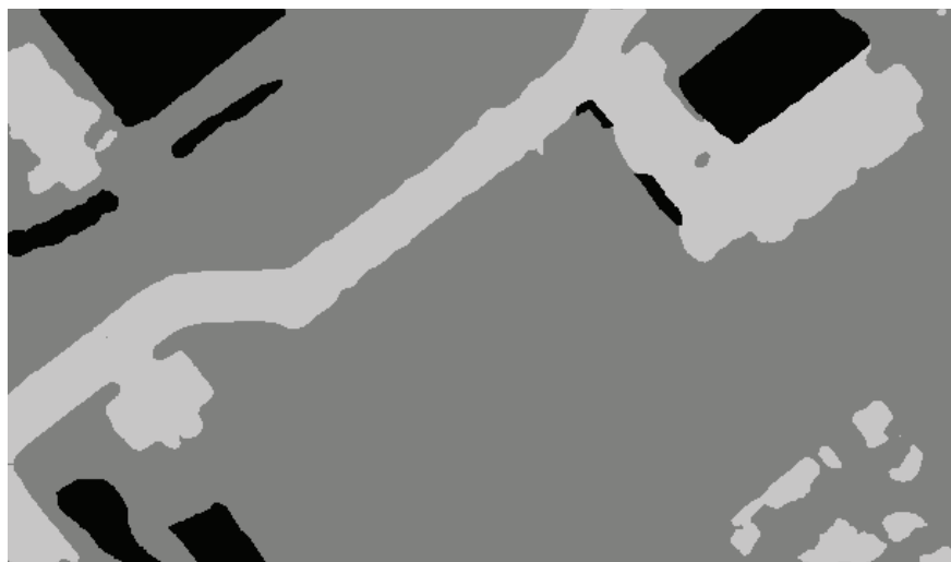
Figure 4.5: Power map image after k-means segmentation. The color variation represents the traversability of the area. [7]
