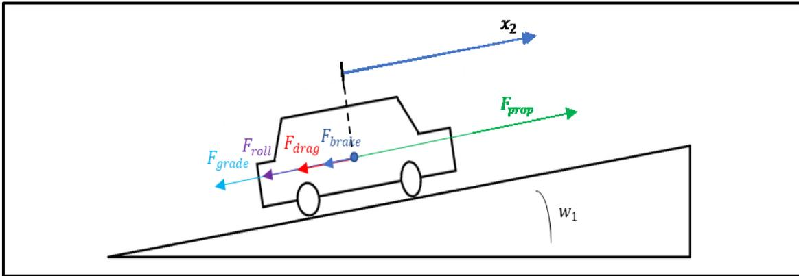
**Figure 2. Free-Body Diagram of Longitudinal Dynamics Model**
