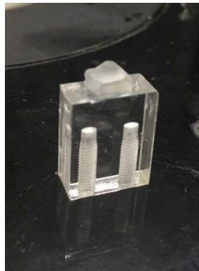
Figure 6. Rectangular prism load cell attachment
