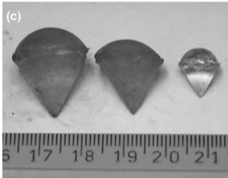
Figure 5. Conical clots used in experimental and computational study by Stewart et al. 8
