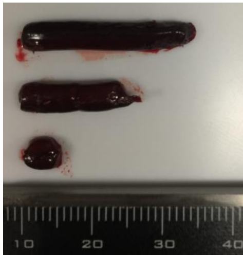
Figure 14. Examples of the bovine whole blood cylindrical clots. Sizes are 5.3 mm 5D (top), 5.3 mm 3D (middle), and 5.3 mm 1D (bottom).
