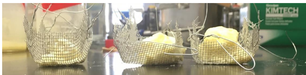
Figure 4.4: Model chocolate samples after hexane immersion. (12 \mu\text{m} sucrose, 40% sucrose, 0% water, left; 40% sucrose, 1% water, middle; 40% sugar, 10% water, right)
