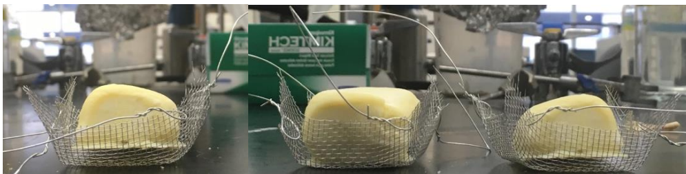
Figure 4.1: Model chocolate samples before hexane immersion. (60 \mu\text{m} sucrose, 20% sucrose, 0% water on left; 20% sucrose, 1% water middle; 40% sucrose, 10% water right)
