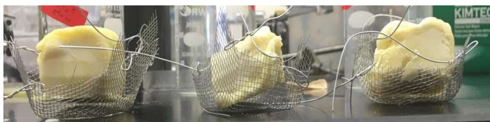
Figure 4.3: Model chocolate samples before hexane immersion. (12 \mu\text{m} sucrose, 40% sucrose, 0% water, left; 40% sucrose, 1% water, middle; 40% sugar, 10% water, right)
