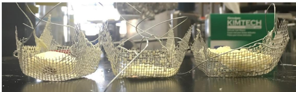
Figure 4.2: Model chocolate samples after hexane immersion. (60 \mu\text{m} sucrose, 20% sucrose, 0% water on left; 20% sucrose, 1% water middle; 40% sucrose, 10% water right)
