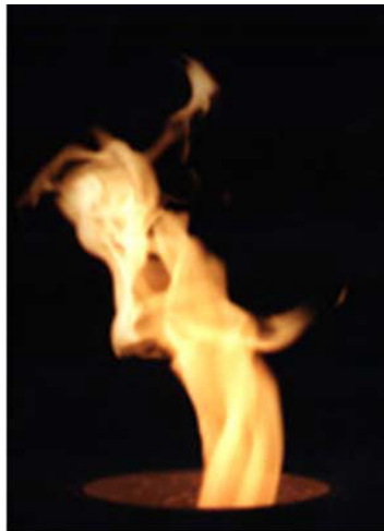
Figure 6: PVC visualization in a reacting flow [15]
