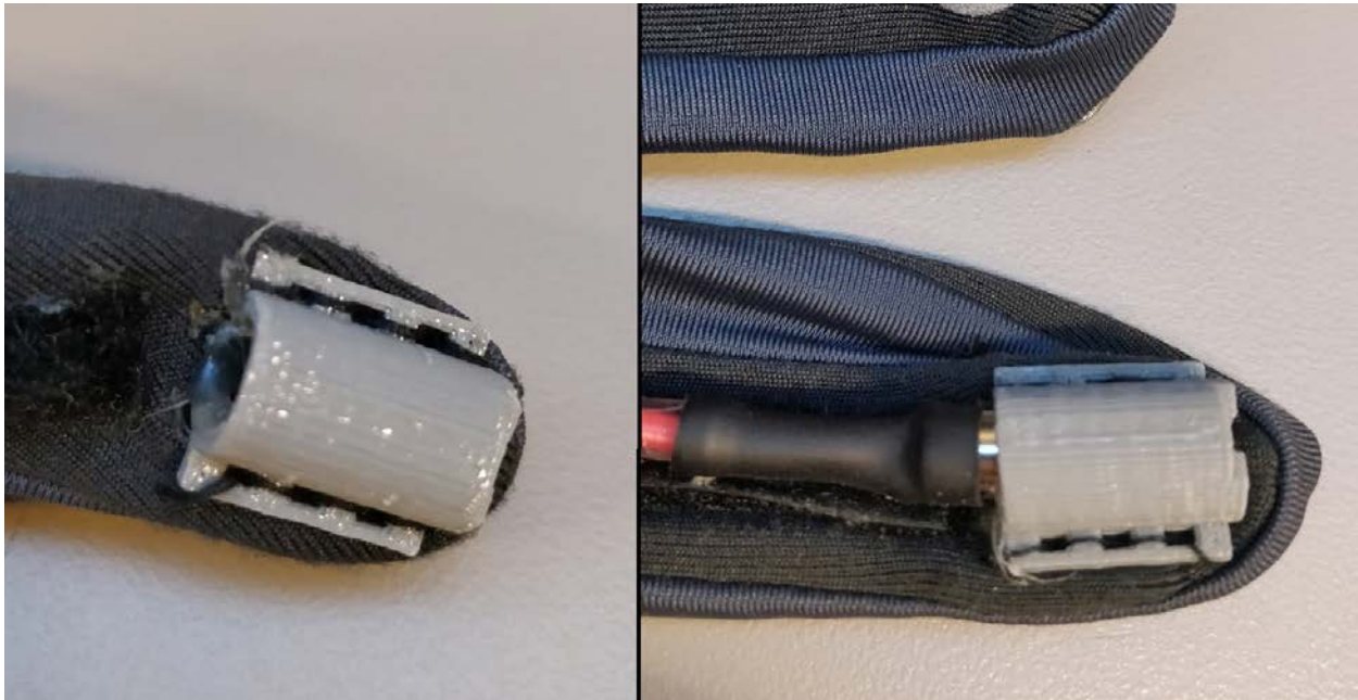
Figure 6. Motor Housing (Left) and the Motor Inside the Housing (Right)
