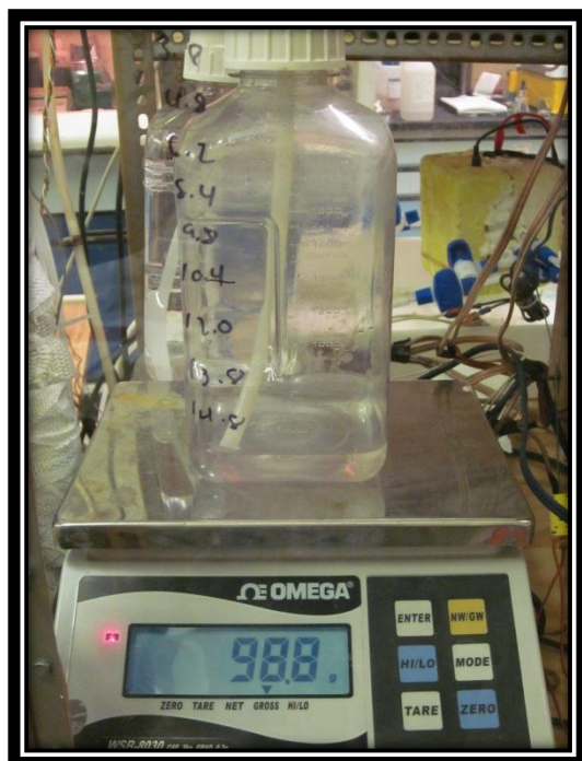
Figure A-8: The water tub was placed on top scale. Any H 2 produced was sent to this tub.
