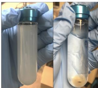
Figure 4. 25% Octyl-POE solution and OmpF protein before and after ultra-centrifugation
