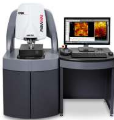
Figure 3.4 Zygo Nextview 3D Optical Profilometer. 41
