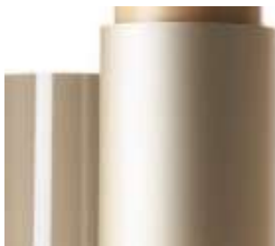
Figure 3.3 Raw PEEK film purchased from Victrex APTIV. 40
