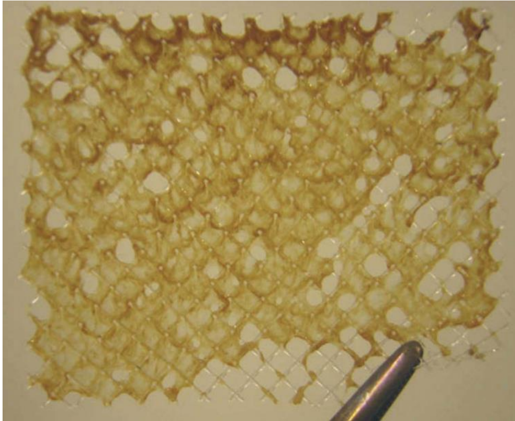
Figure 5. Biofilm growth within the matrix of the feed spacer 18
