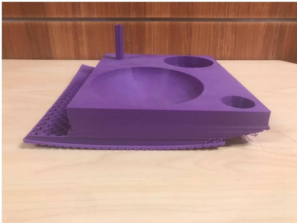
Figure 2: Effect of Warping on a 3D Printed Part
