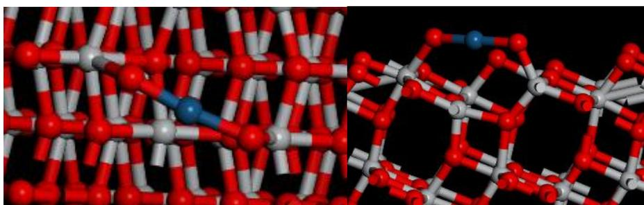
Figure 16a/16b: Top and side view of bare PtO/TiO<sub>2</sub> surface
