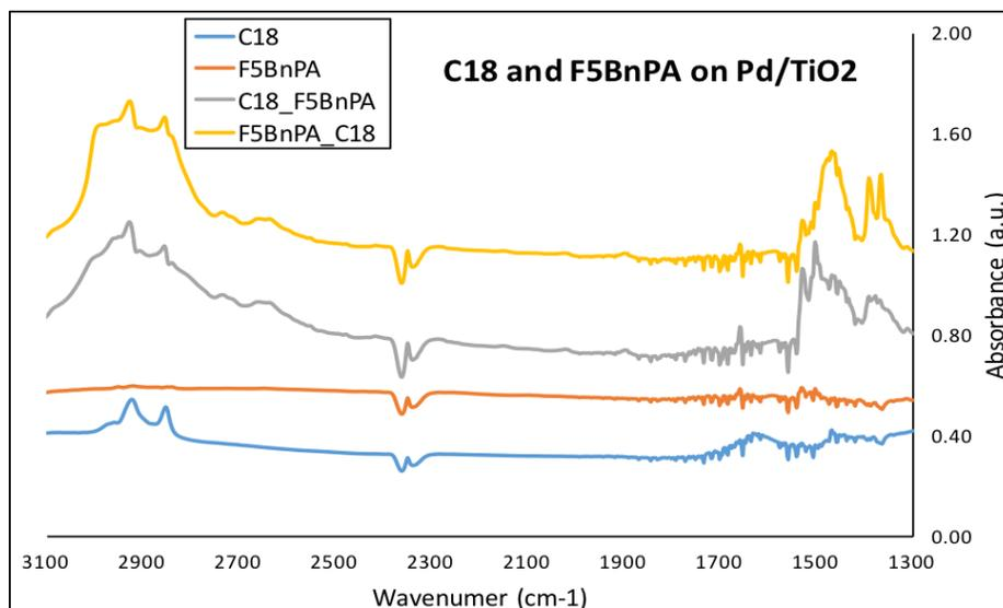
Figure 5: F5BnPA and C18 both are on the surface when the support is changed to titania.
