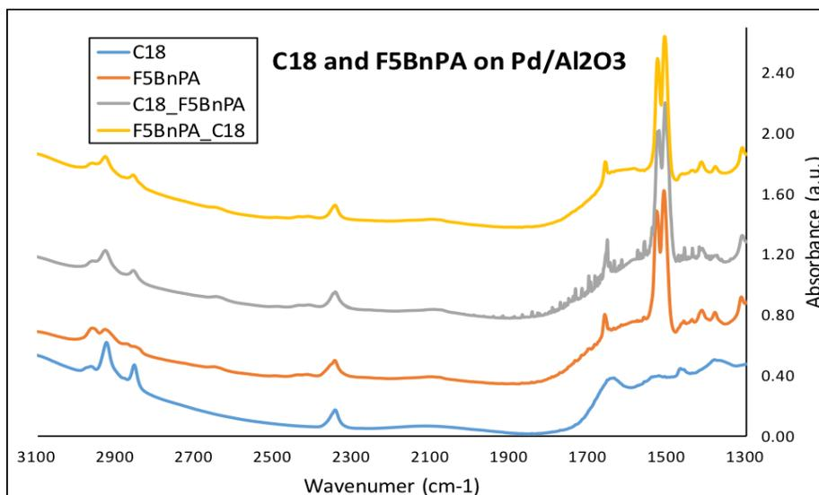
Figure 3: IR data for the thiol, C18, and phosphonate, F5BnPA, added to the surface of a Palladium catalyst separately and in combination.
