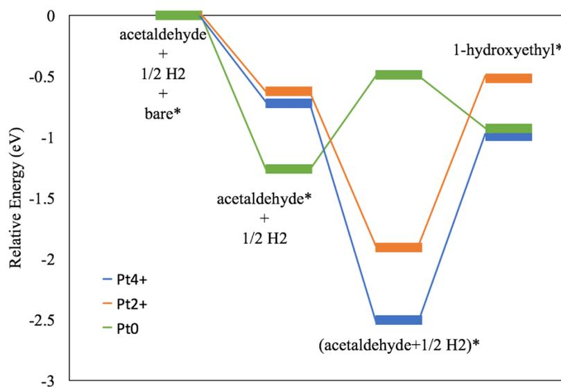
Figure 21: Relative energy comparison of reaction pathway for acetaldehyde hydrogenation
