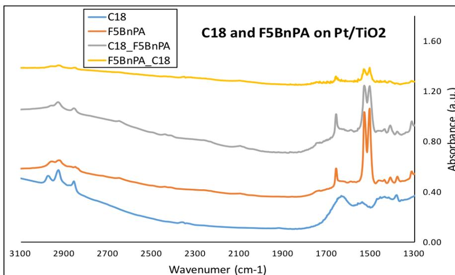
Figure 6: Signals were somewhat weak, but the thiol and phosphonate are visible on the spectra.
