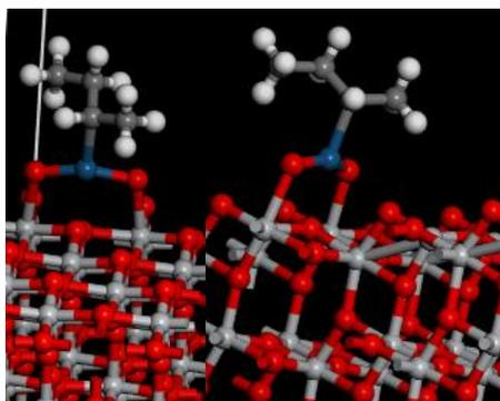
Figure 23a/23b: Hydrogenated trans-2-butene (trans-2-butyl) adsorbed on PtO<sub>2</sub>/TiO<sub>2</sub>
