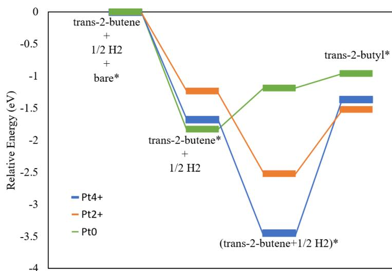
Figure 20: Relative energy comparison of reaction pathway for trans-2-butene hydrogenation
