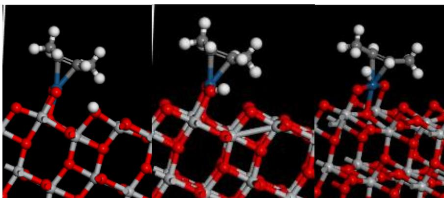
**Figure 22a/22b/22c: Hydrogen adsorbed on surface oxygen, added oxygen, and Pt atom**
