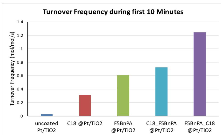
Figure 13: Overall turnover frequency on titania supported catalysts.
