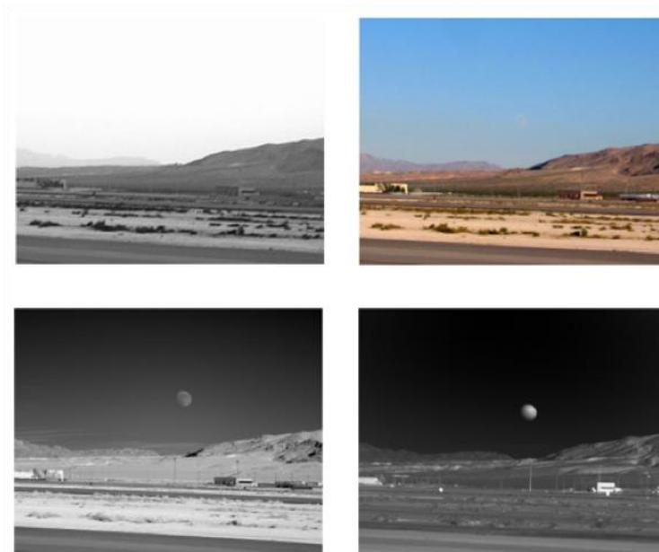
Figure 10: Images in near UV, VIS, NIR, MIR (reading left to right) [25].
