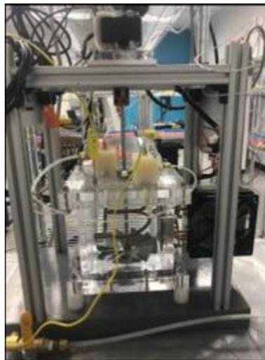
**Figure 4 Thermal mass with mounted Peltier cooler**
