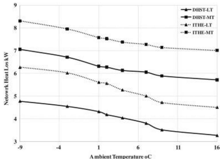
Figure 2 Effects of Ambient Temperature on Heat Loss [4]
