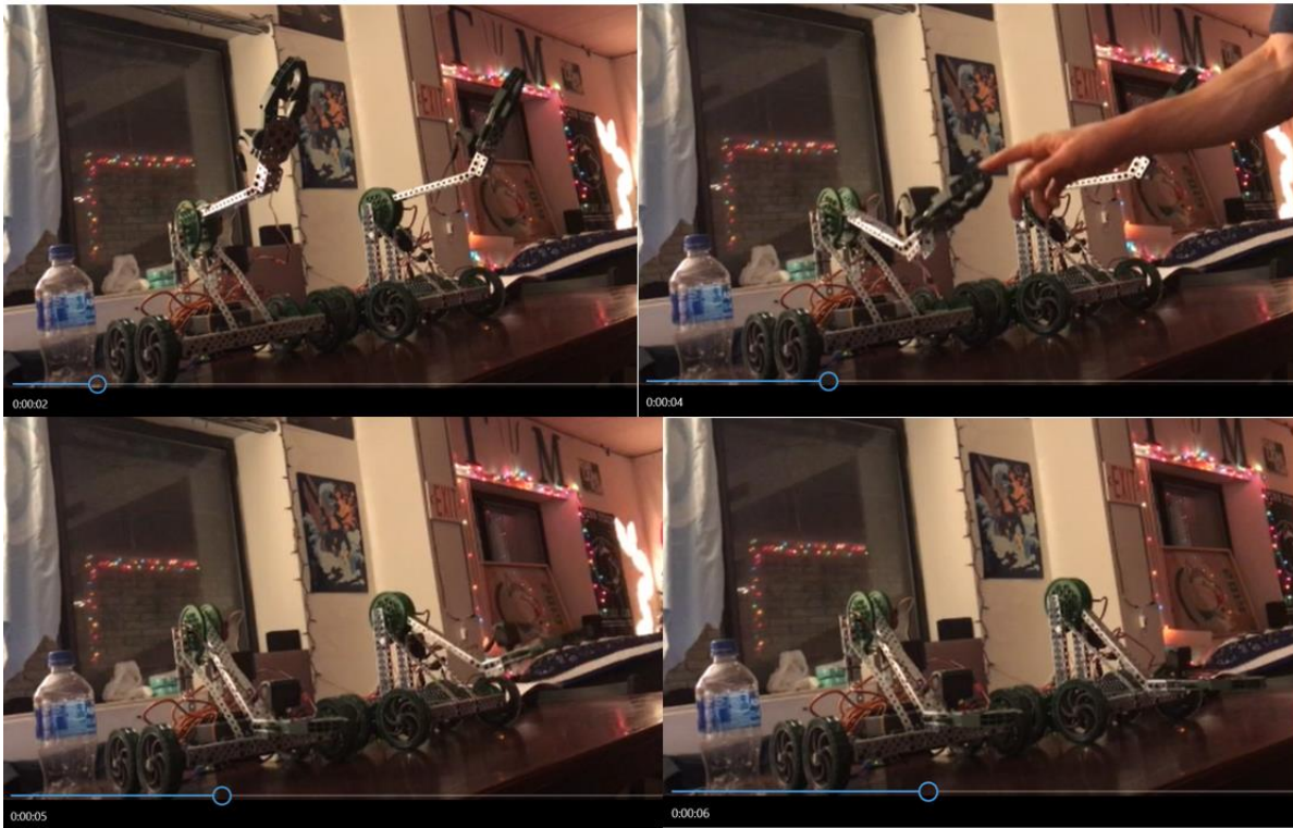
Figure 11. Time stamps for arm movement of Original (left) and Copy (right). Close inspection reveals a slight time delay between the two but accurate speed and position. Left to right and top to bottom the time stamps are as follows: t = 2\text{s} , 4\text{s} , 5\text{s} , and 6\text{s} .
